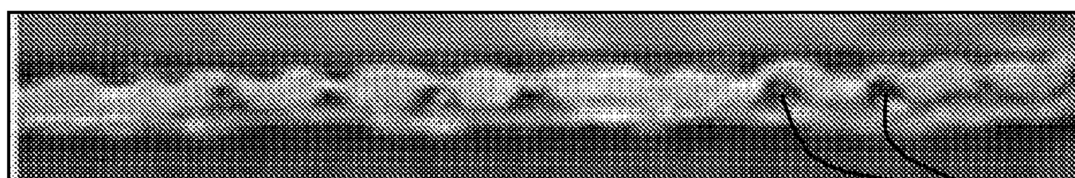
8% Talc 2 in TPO Thickness = 0.38 mm RWT = 0.11 \pm 0.01 mm
