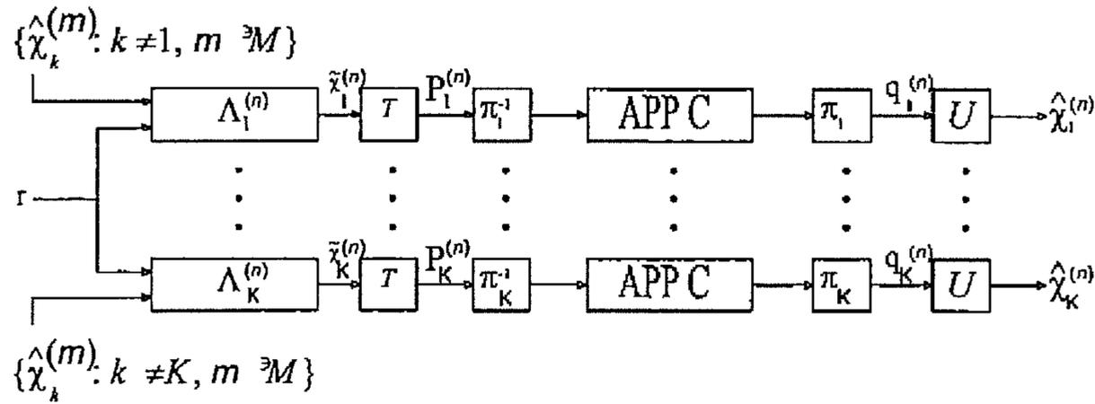
Iterative multiuser decoder with linear multiuser estimation
