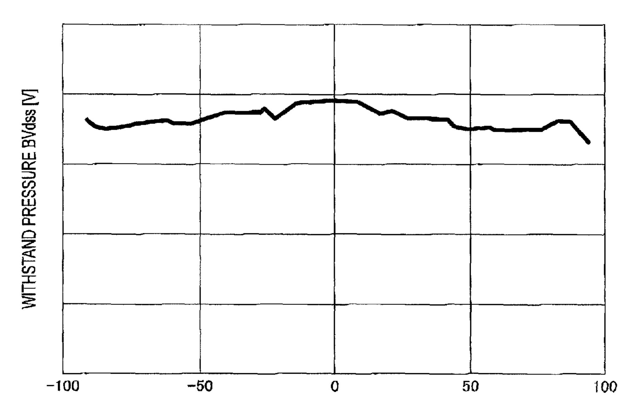
DISTANCE FROM CENTER OF EPITAXIAL SILICON WAFER [mm]
