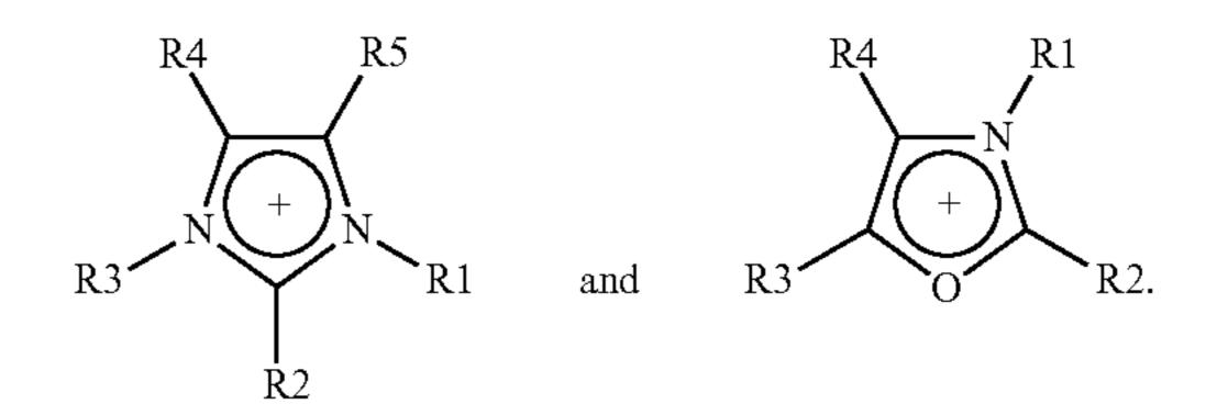
**13**. The method according to claim **1**, wherein the ionic liquids have the general formula (I)
