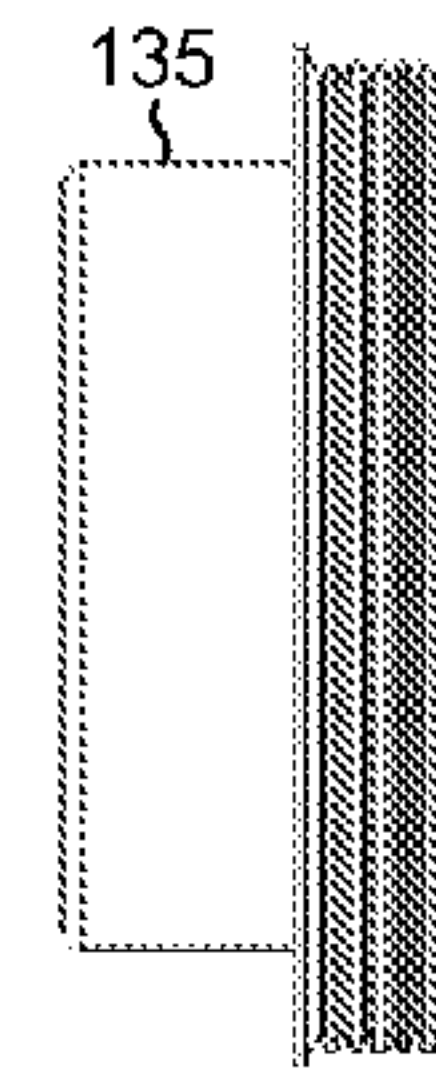
SIDE VIEW OF DRIVE PULLEY
