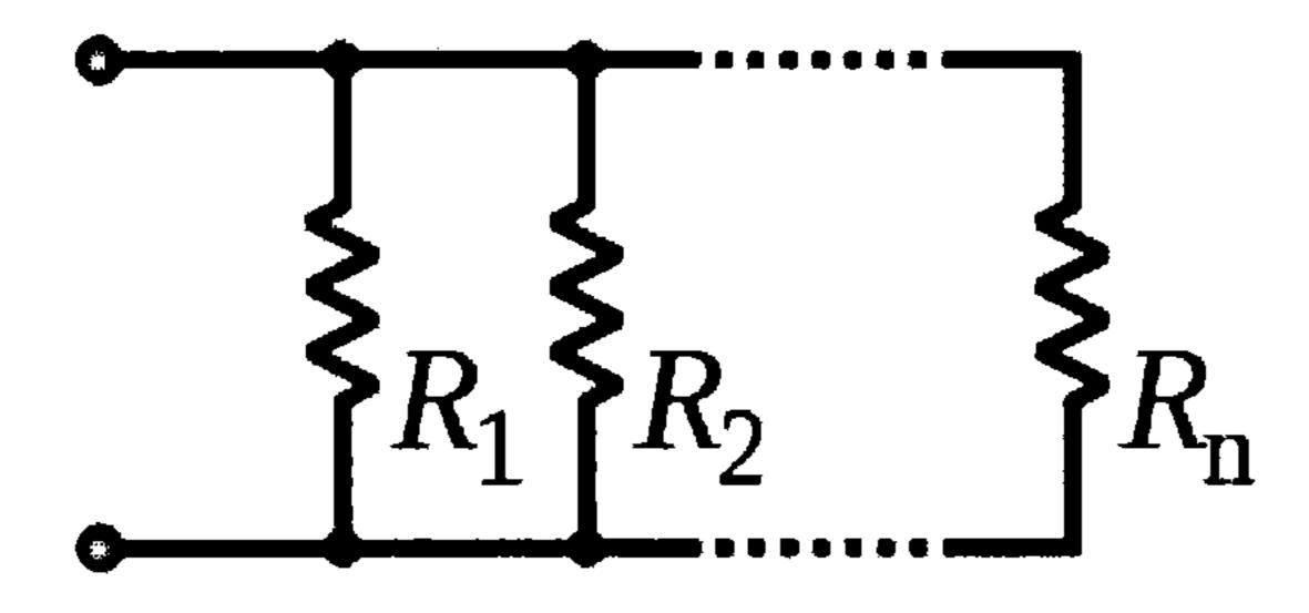
$$\frac{1}{R_{\text{total}}} = \frac{1}{R_1} + \frac{1}{R_2} + \dots + \frac{1}{R_n}$$
