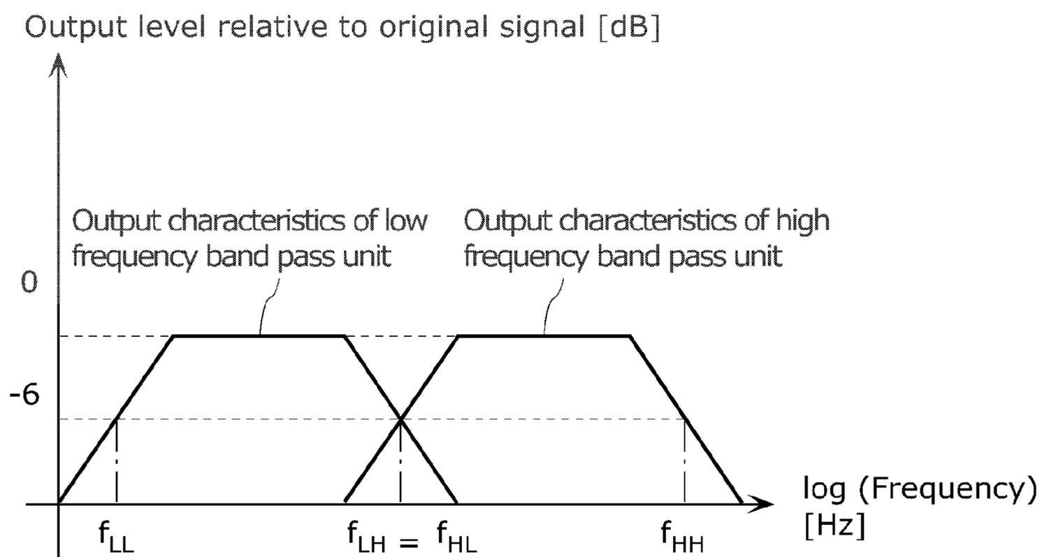
$f_{LL}$  : Lower end of output frequency band of low frequency band pass unit
