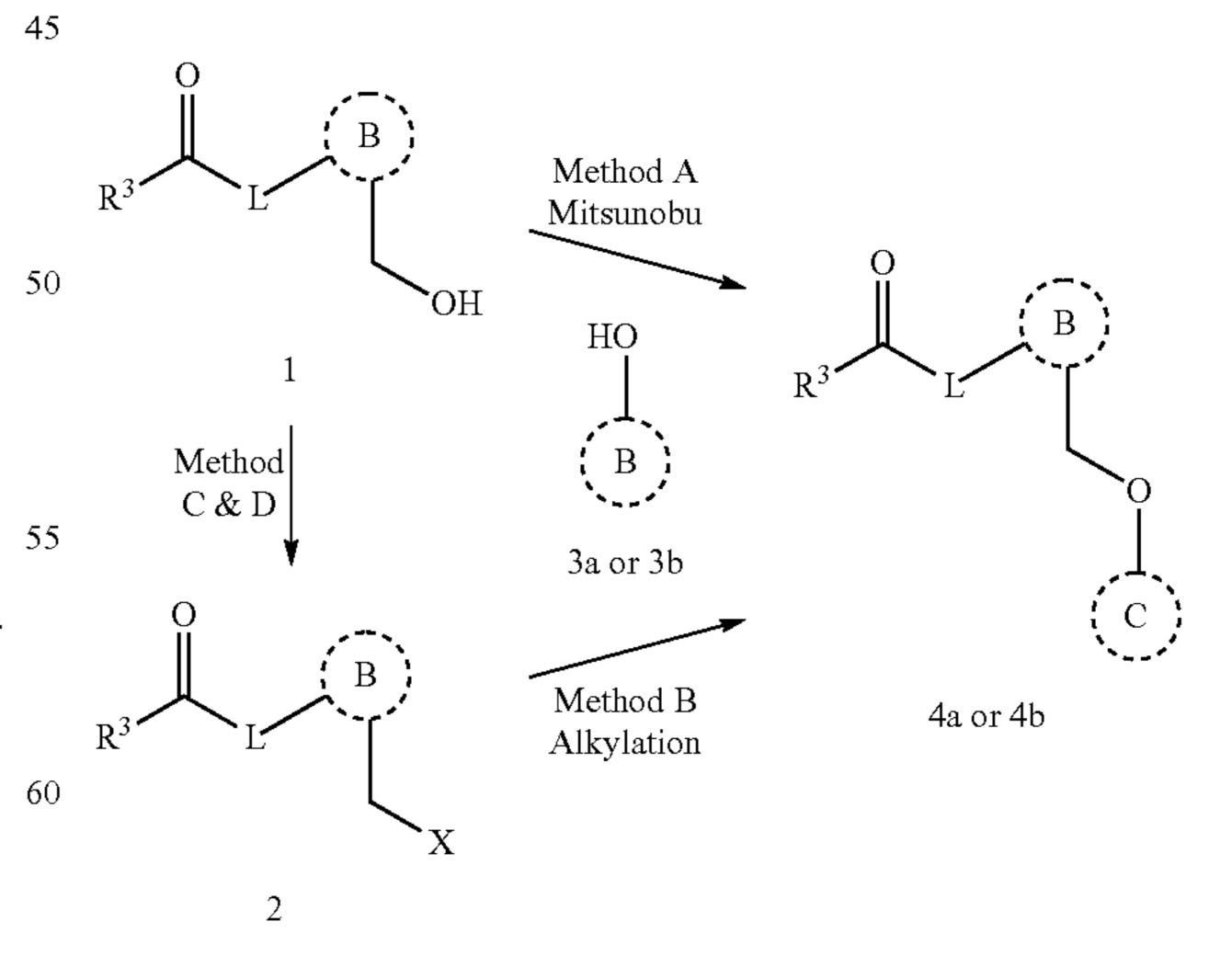
General Method a for Preparing Aryloxy/Heteroarylether Analogs (4a/4b) from Substituted Methylene Alcohol (1) and Hydroxyl (Hetero)Aryl Aldehyde Derivatives (3a/3b).
