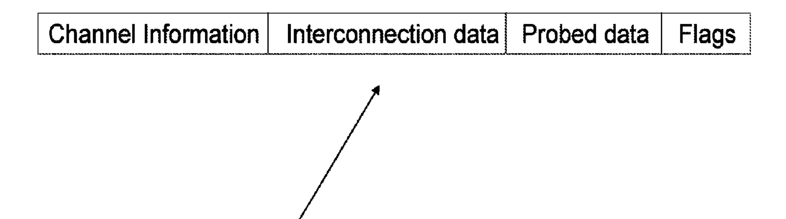
A packet transmitted from a serial transmitting device
