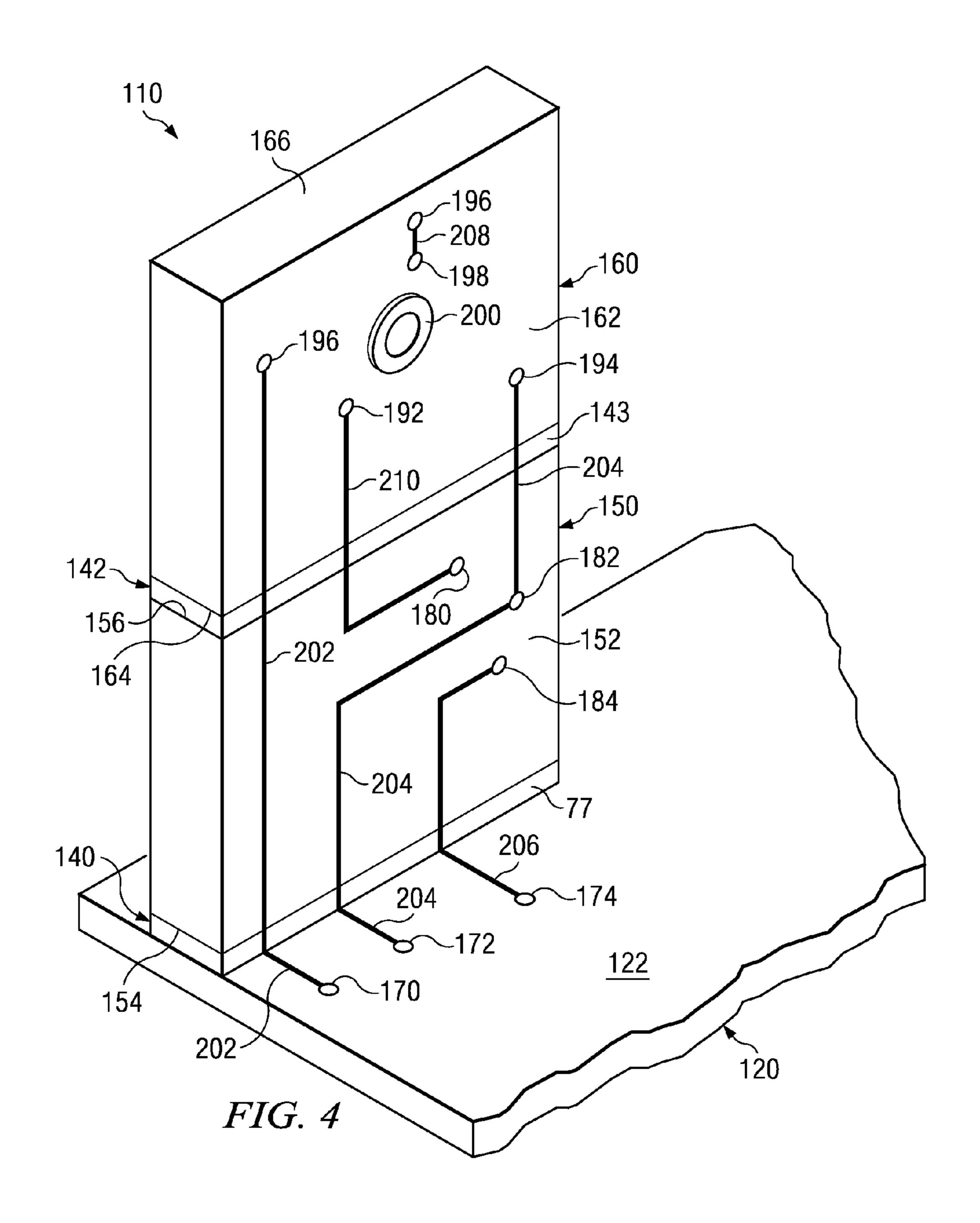
MOUNTING ONE ELECTRICAL SUBSTRATE ON ANOTHER ELECTRICAL SUBSTRATE WITH A FACE SURFACE ON THE ONE SUBSTRATE ORIENTED TRANSVERSELY OF A FACE SURFACE OF THE OTHER SUBSTRATE
