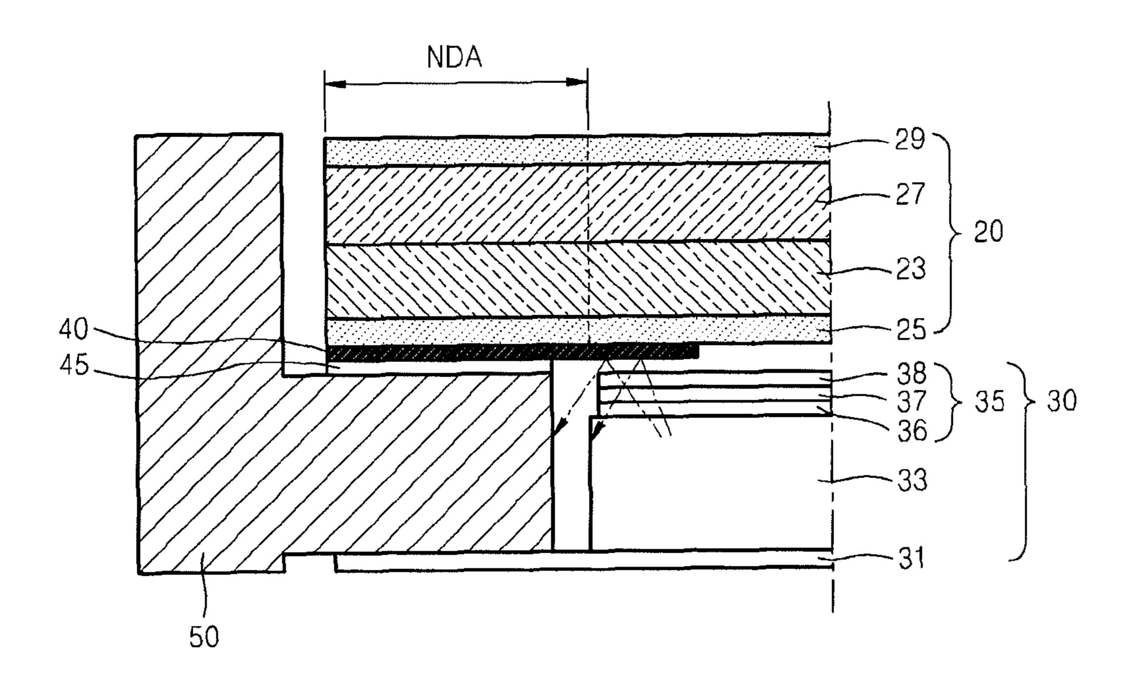
BACKLIGHT ASSEMBLY AND LIQUID CRYSTAL DISPLAY DEVICE INCLUDING THE SAME COMPRISING A SHIELDING TAPE THAT COMPRISES A PORTION HAVING AN ATTACHED ADHESIVE AND A PORTION WITHOUT THE ADHESIVE
