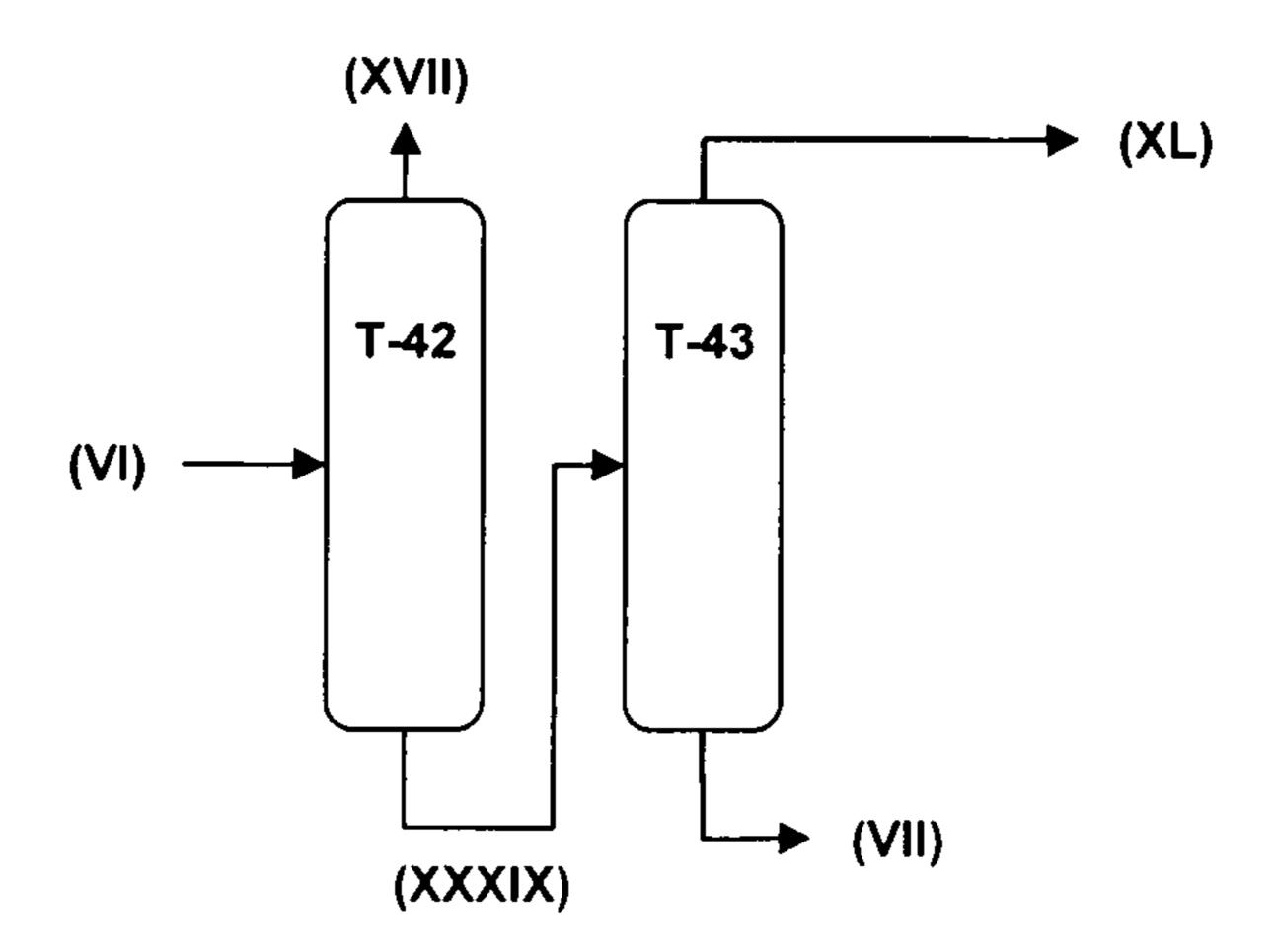
Figure 10: Removal of water, preferred embodiment [e1]
