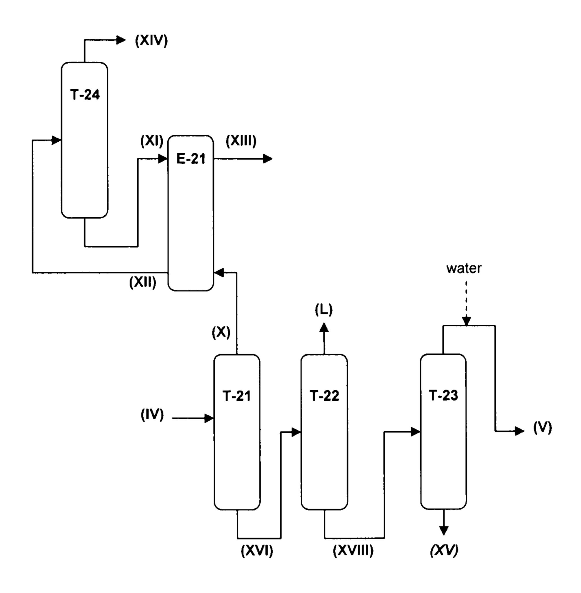
Figure 6: Isolation of MTBE, preferred embodiment [b4]
