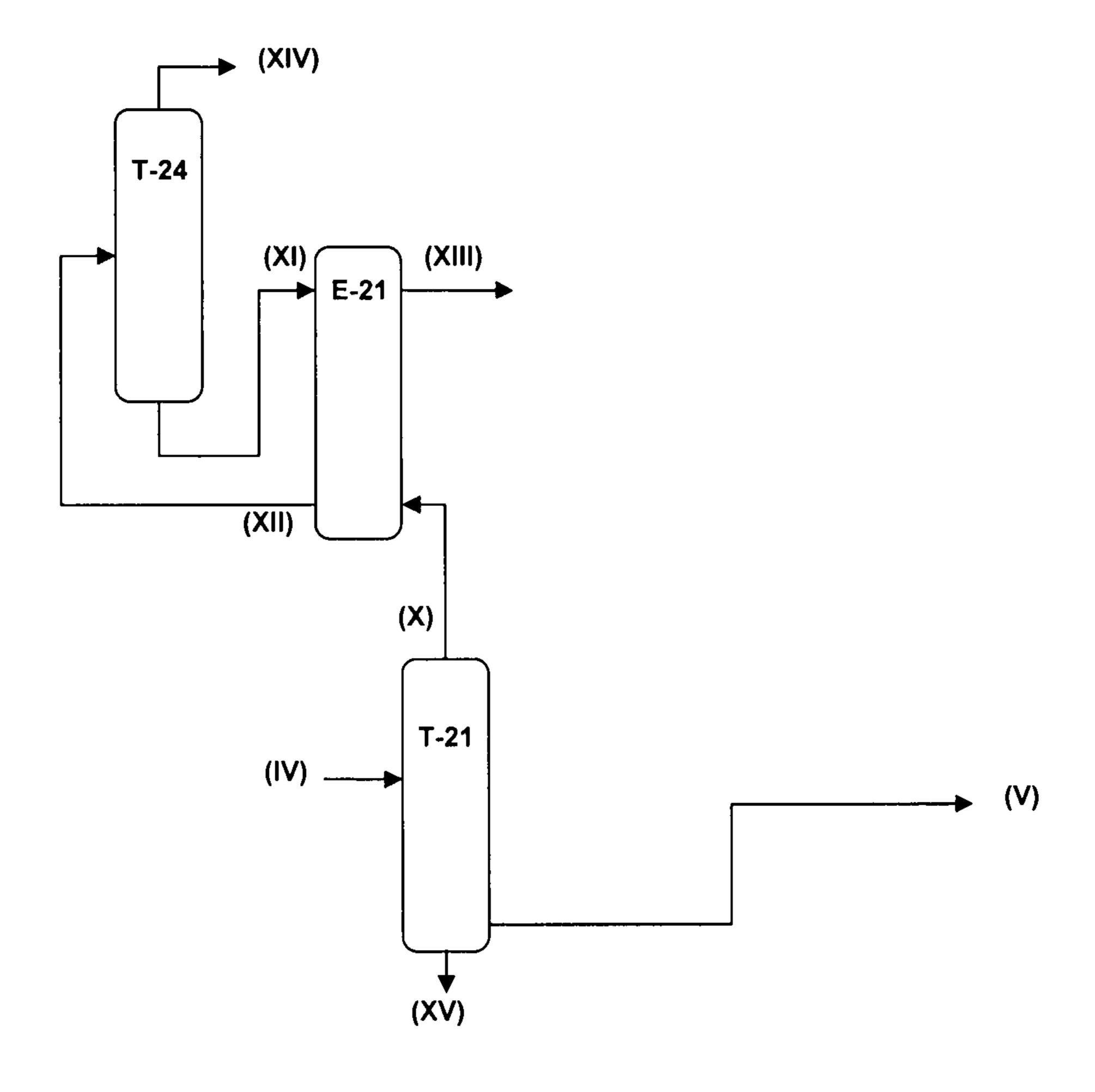
Figure 4: Isolation of MTBE, preferred embodiment [b2]
