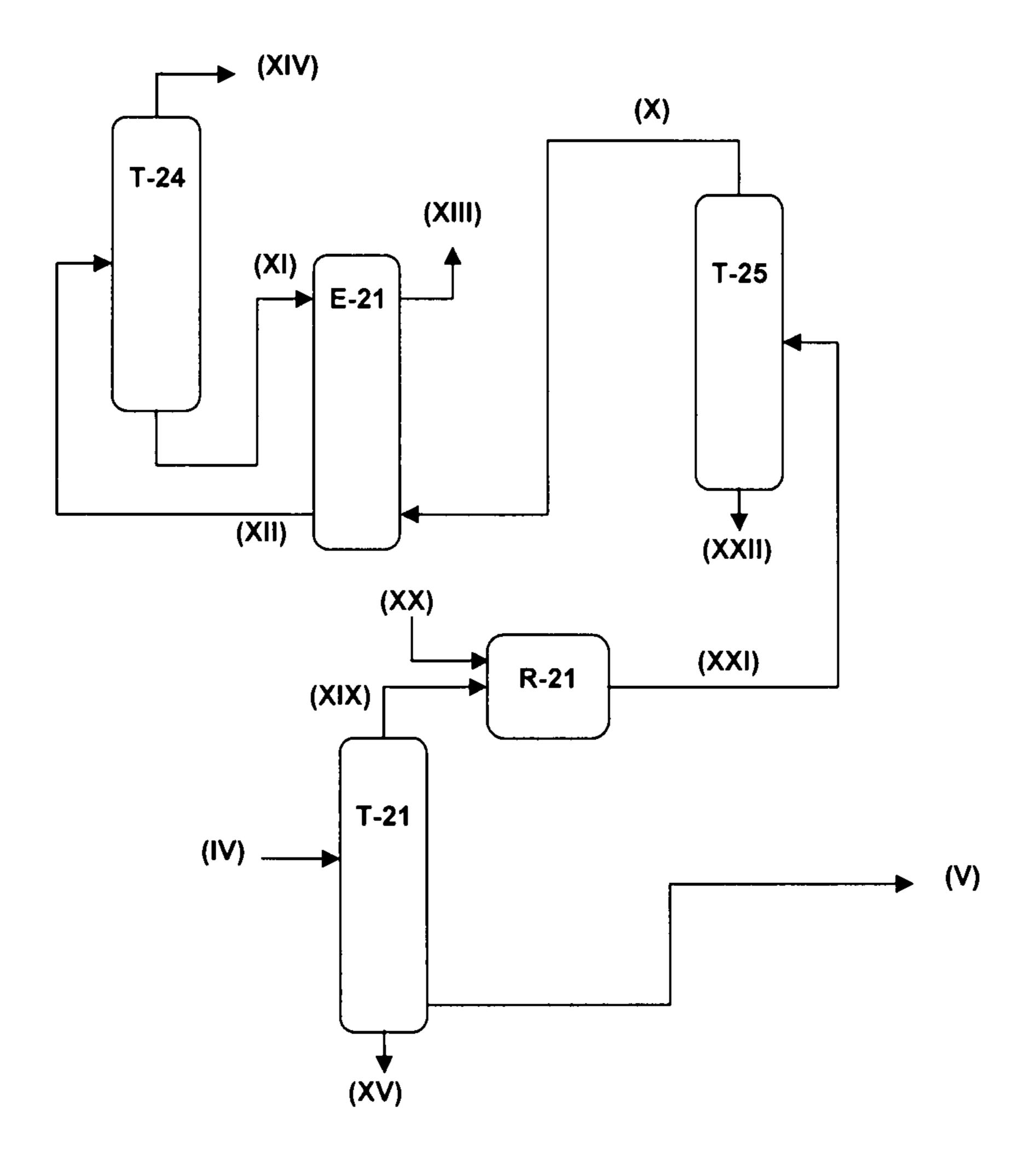
Figure 7: Isolation of MTBE, preferred embodiment [b5]
