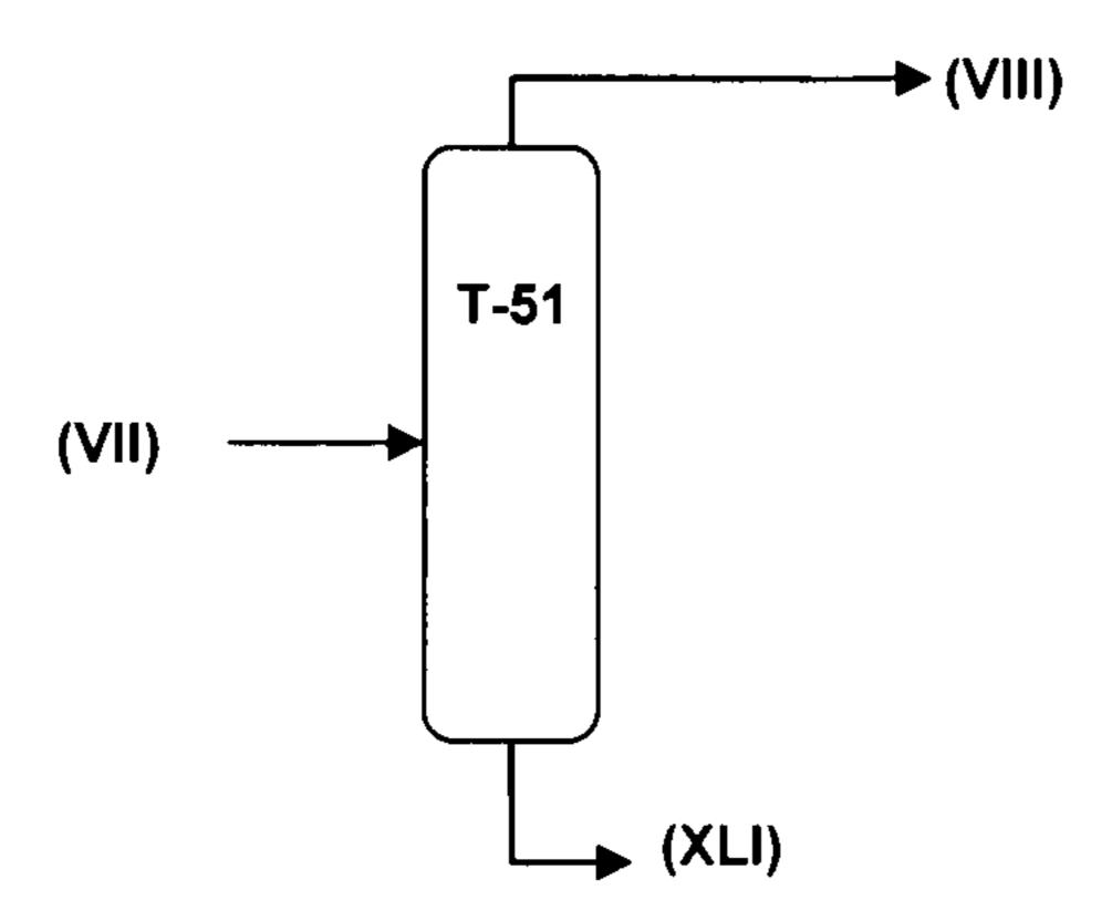
Figure 11: Removal of water, preferred embodiment [e2]
