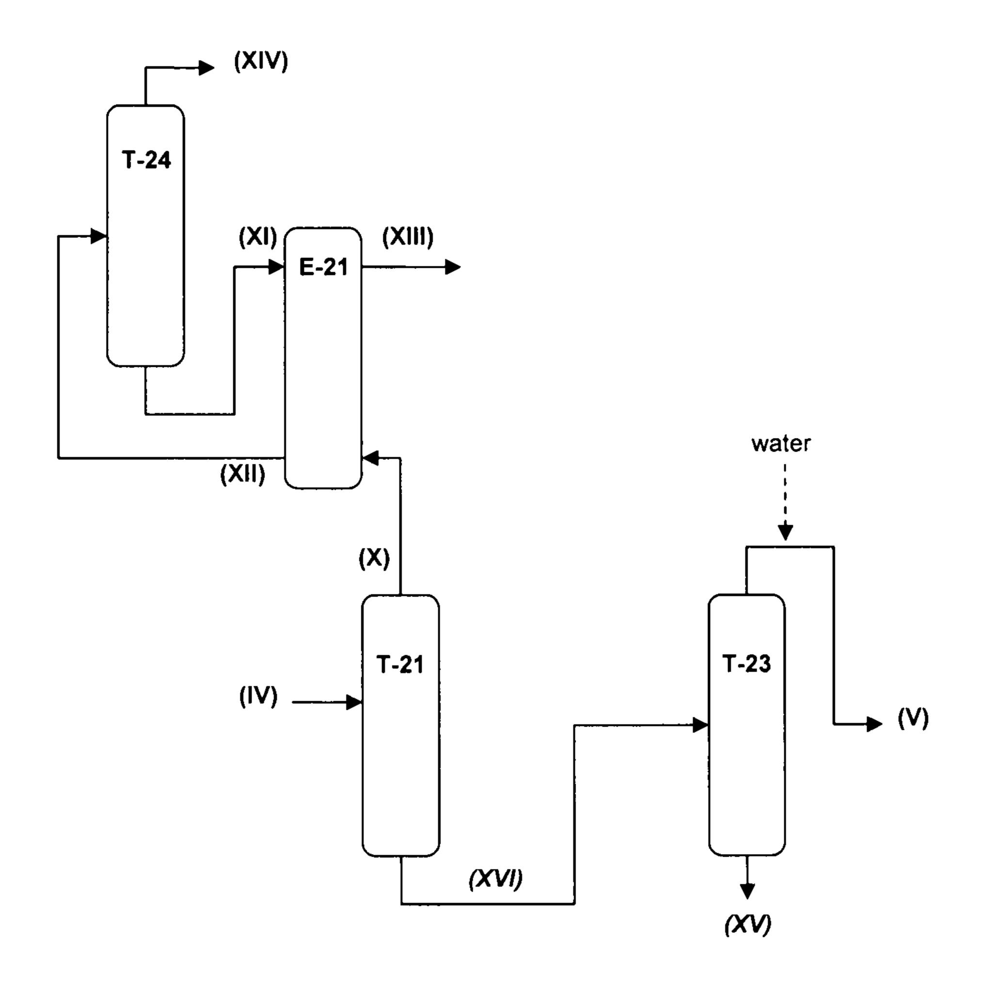
Figure 5: Isolation of MTBE, preferred embodiment [b3]
