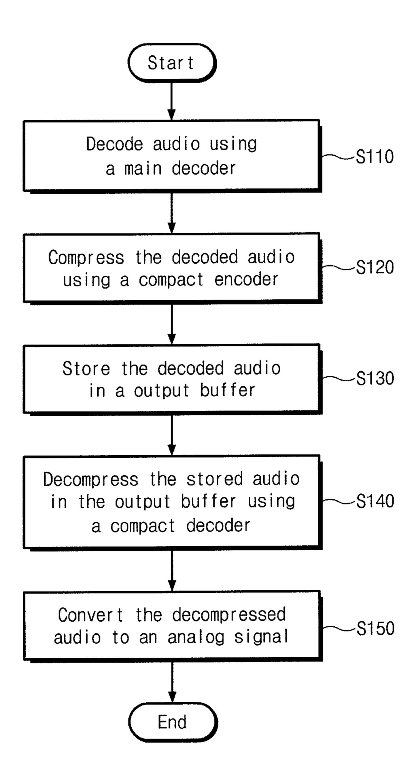
AUDIO DECODING SYSTEM AND AN AUDIO DECODING METHOD THEREOF FOR COMPRESSING AND STORING DECODED AUDIO DATA IN A FIRST TIME INTERVAL AND DECOMPRESSING THE STORED AUDIO DATA IN A SECOND TIME INTERVAL
