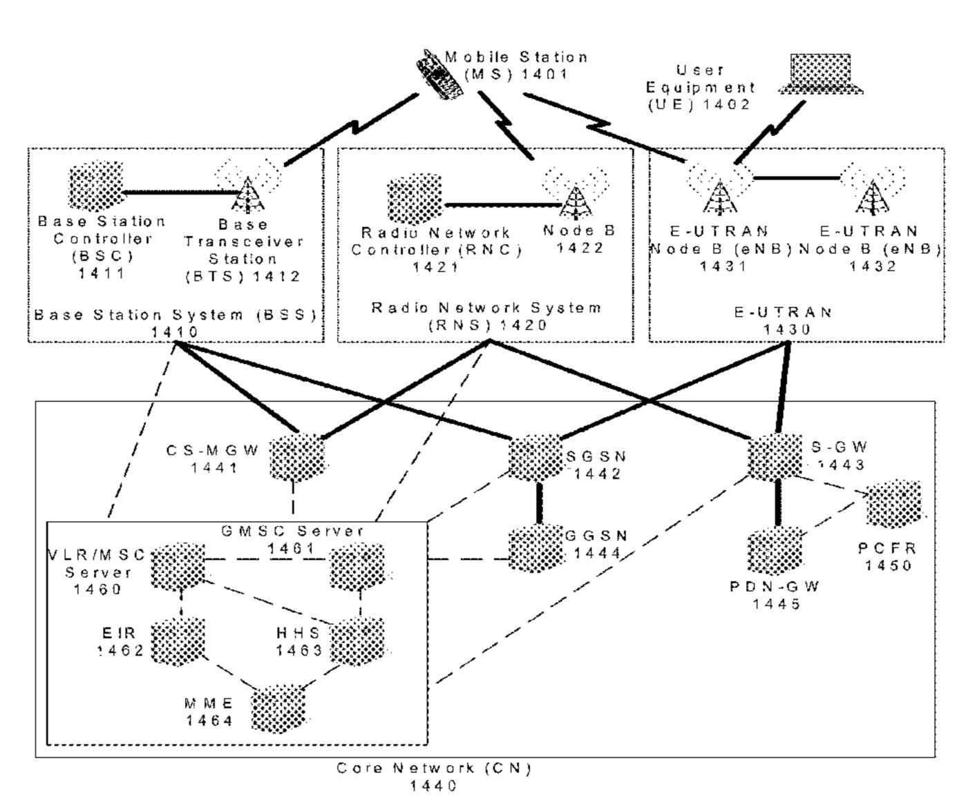
\*NOTE Solid Lines represent user traffic signals while dashed lines represent support signaling
