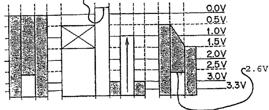
FIG. 14A  $t_4 < t < t_5$  TRANSFER OF STORED CHARGES FROM PD TO FD
