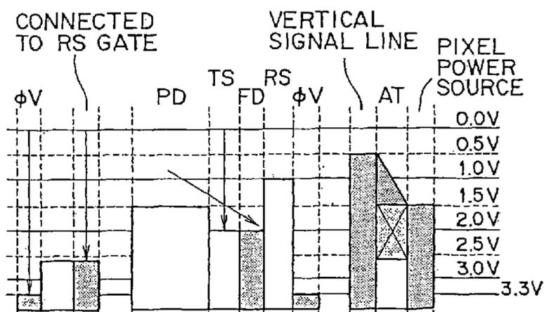
FIG. 14B  $t_5 < t < t_6$  SIGNAL LEVEL READ-OUT
