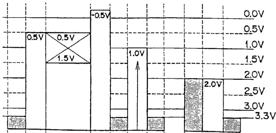
FIG. 5A  $t_3 < t < t_4$  TRANSFER OF SIGNAL CHARGE FROM PD TO FD
