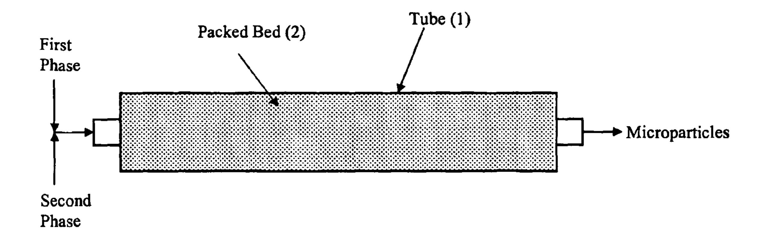
Figure 2 – A Typical Packed Bed Emulsification System
