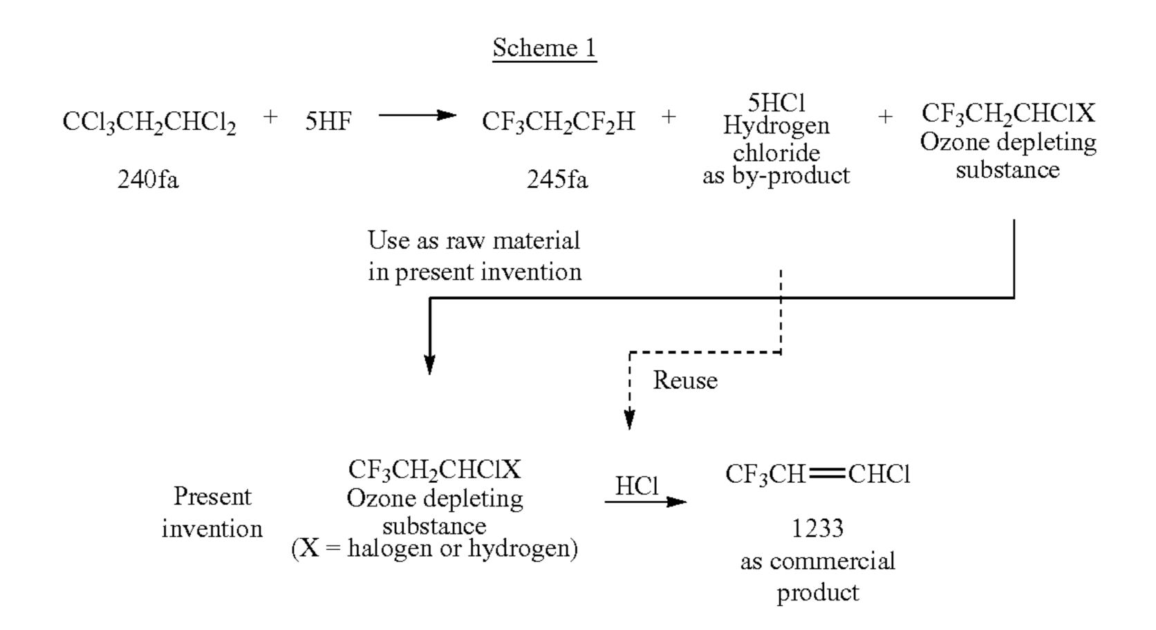
containing a compound of the general formula (1): CF<sub>3</sub>—CHCIX (where X is a fluorine atom or a chlorine atom) into contact with a solid catalyst in the presence of hydrogen chloride. The production method of the present invention is characterized in that the 1233 can be produced selectively 30 with substantially no generation of 1234 as a by-product even though the contact reaction is performed in the presence of hydrogen fluoride.
