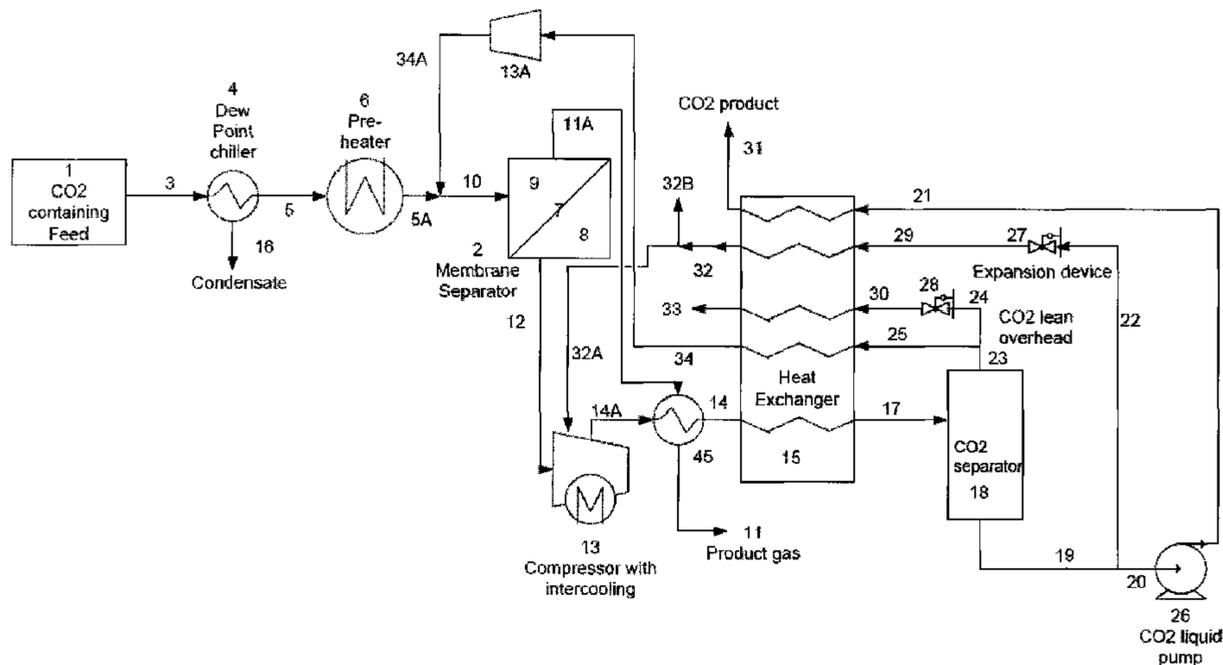
General scheme for membrane + heat exchanger + CO2 separator
