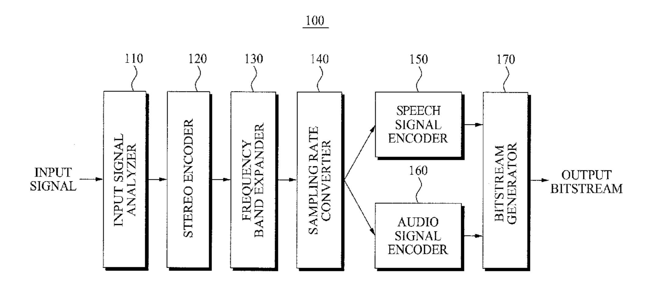
mono signal when the input signal is a stereo signal, and to extract stereo sound image information; a frequency band expander to expand a frequency band of the input signal; a sampling rate converter to convert a sampling rate; a speech signal encoder to encode the input signal using a speech encoding module when the input signal is a speech charac-
