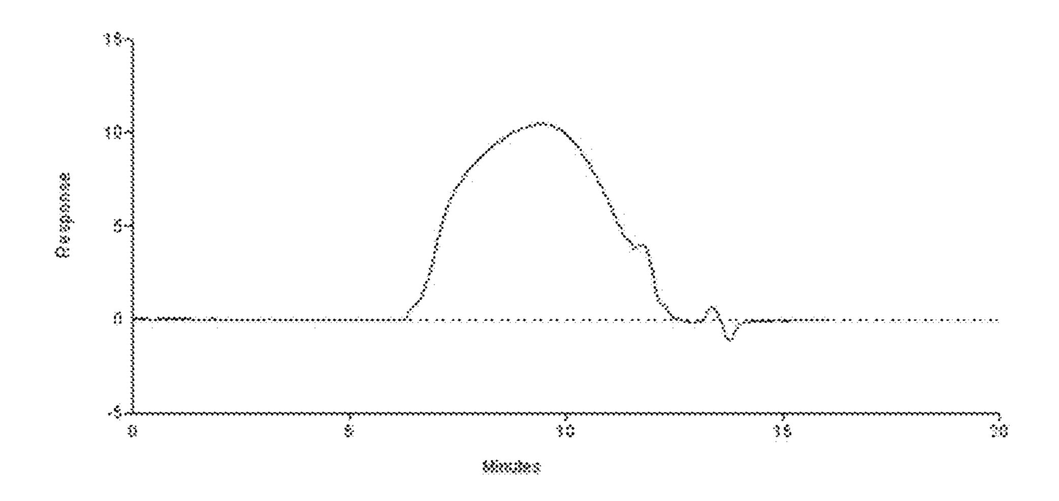
Molecular weight distribution of PTTS formed using (NHC)<sub>2</sub>PdCl<sub>2</sub>; Mw=1580, Mn = 934
