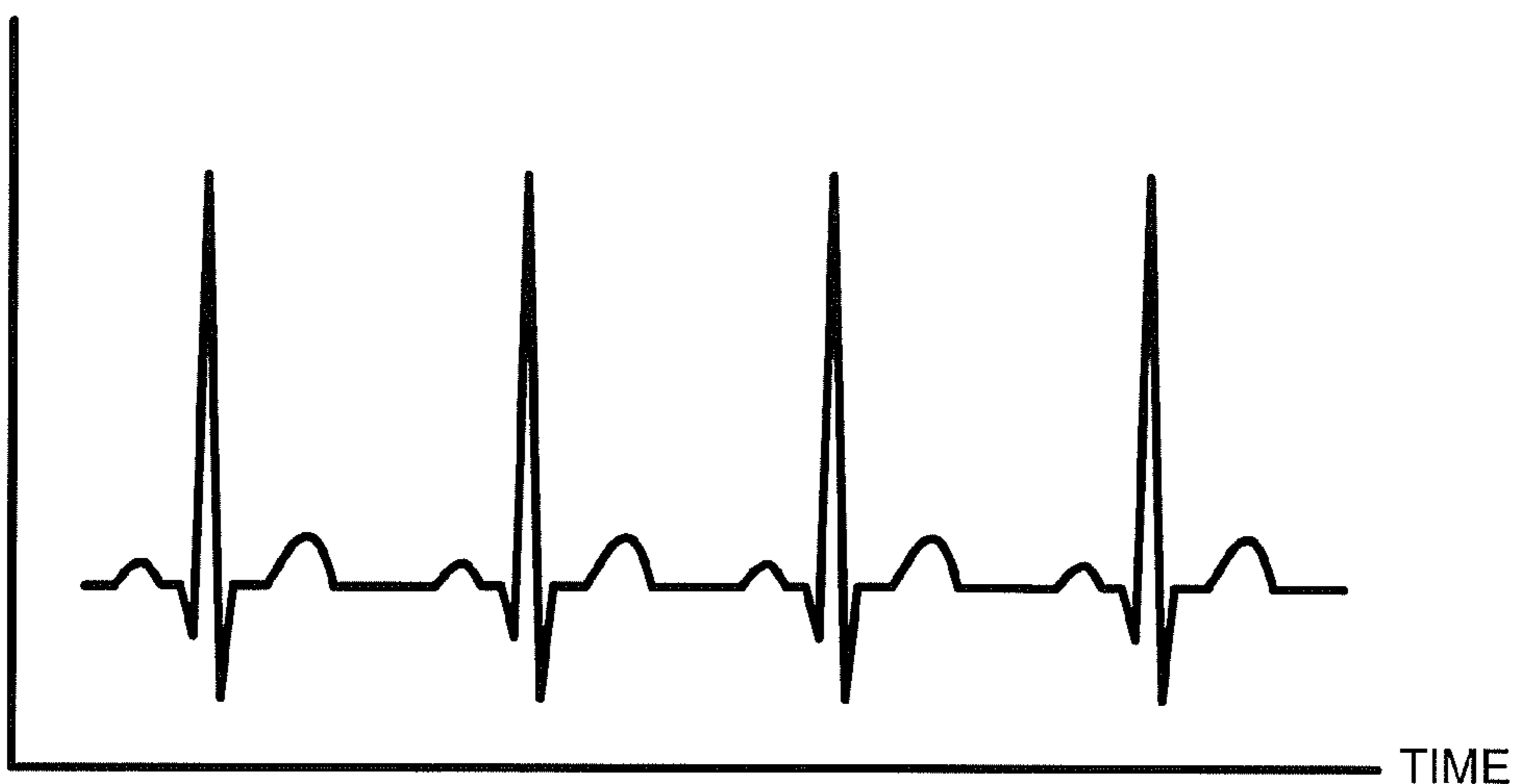
FIG. 6 SAMPLE ECG SIGNAL HAVING QRS COMPLEXES AND NO IMPULSIVE ARTIFACTS
