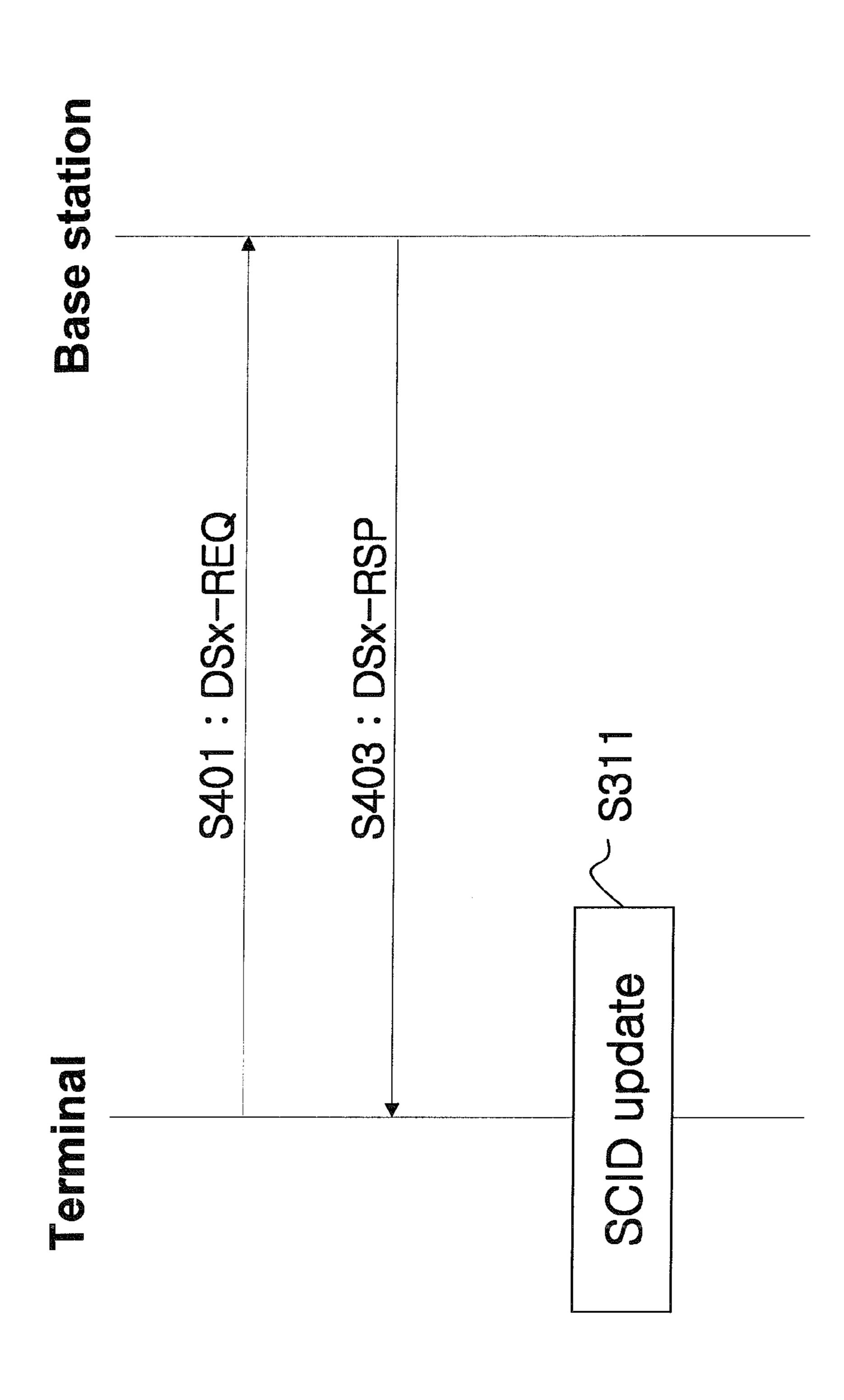
SCID switching through SCEH of DSx-ACK
