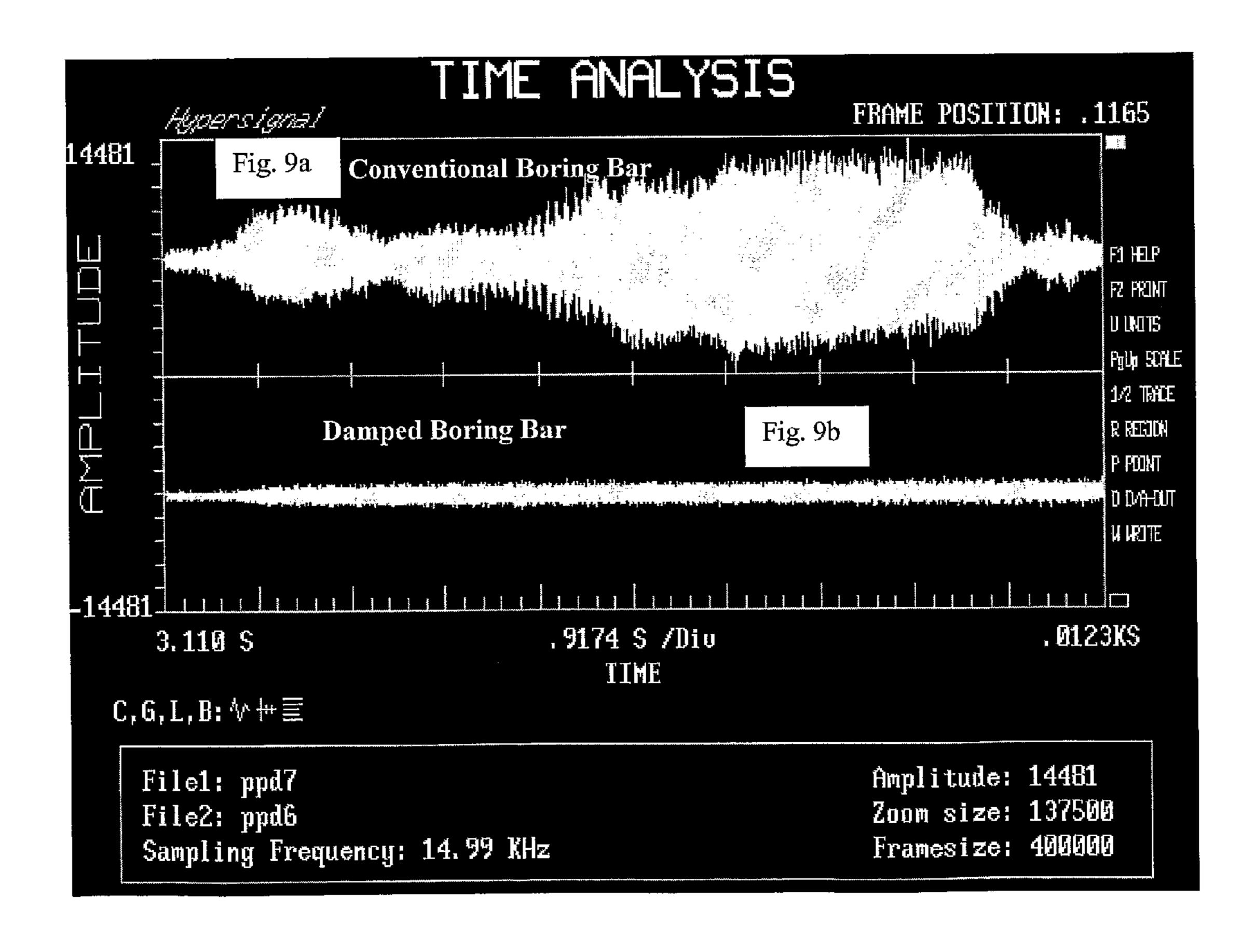
Noise record from machining with conventional boring bar and damped boring bar
