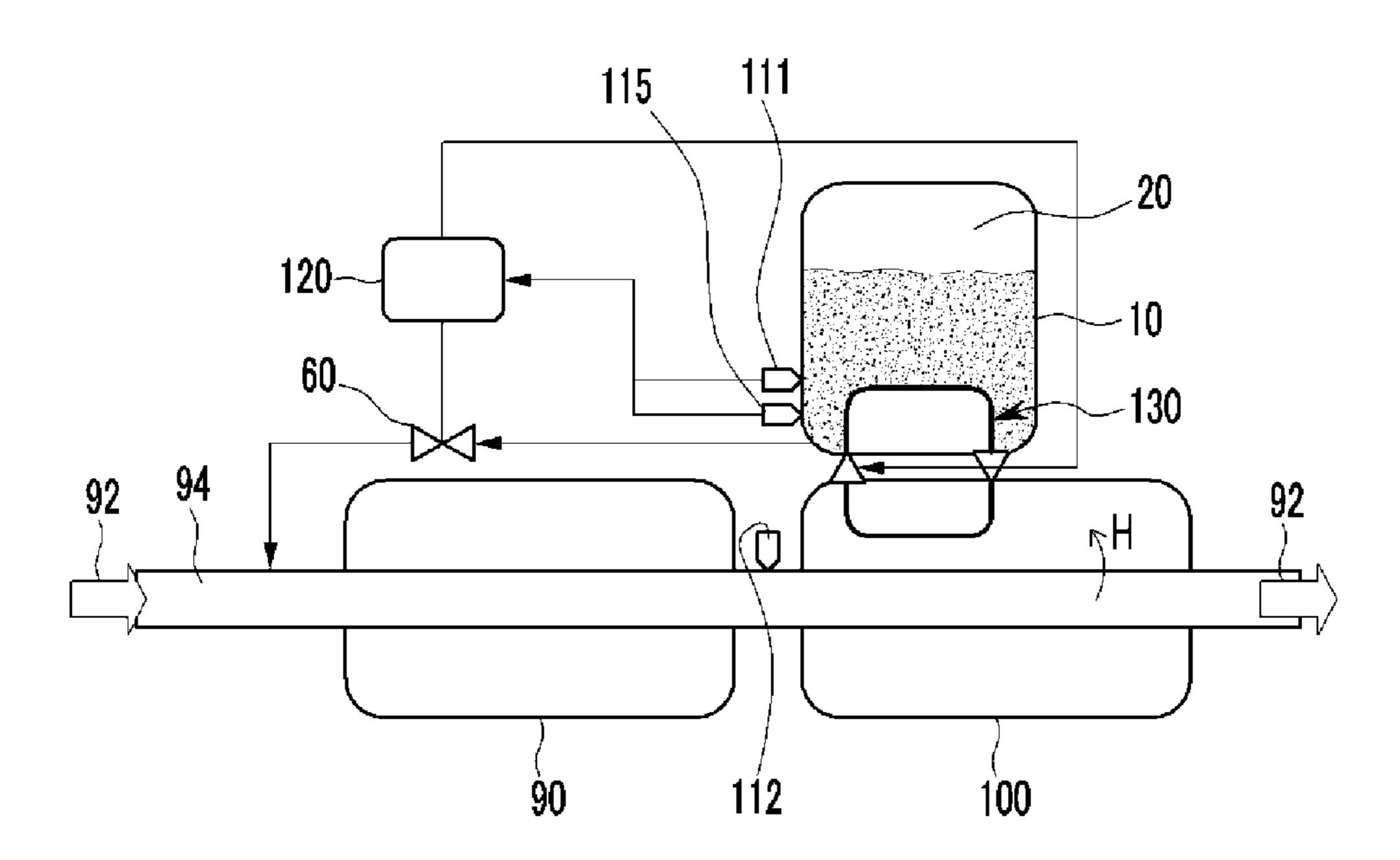
Heat exchange lexhaust heat recovery device in \
