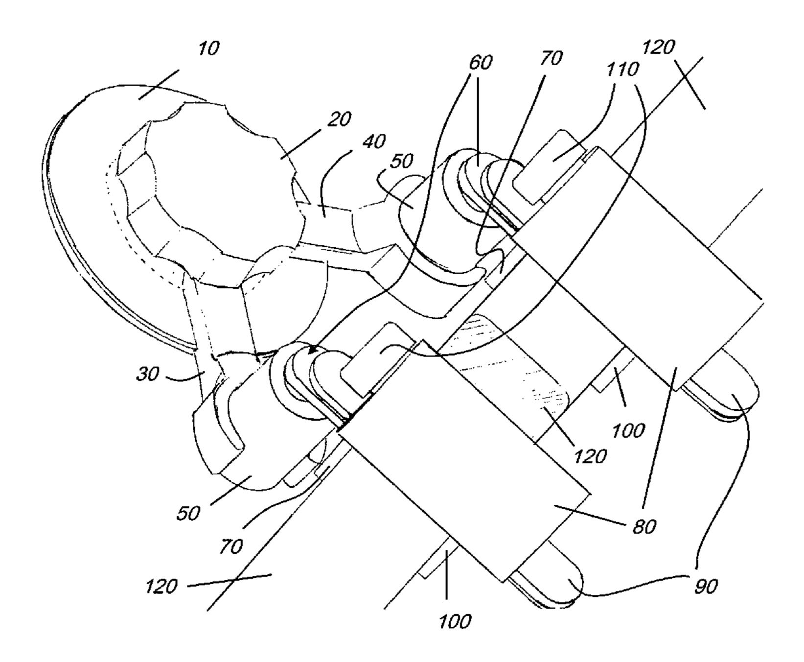
Caricature of an upper view of an illustrative, non-exclusive embodiment of a device according to the invention when locking windshield wipers on a vehicle window.
