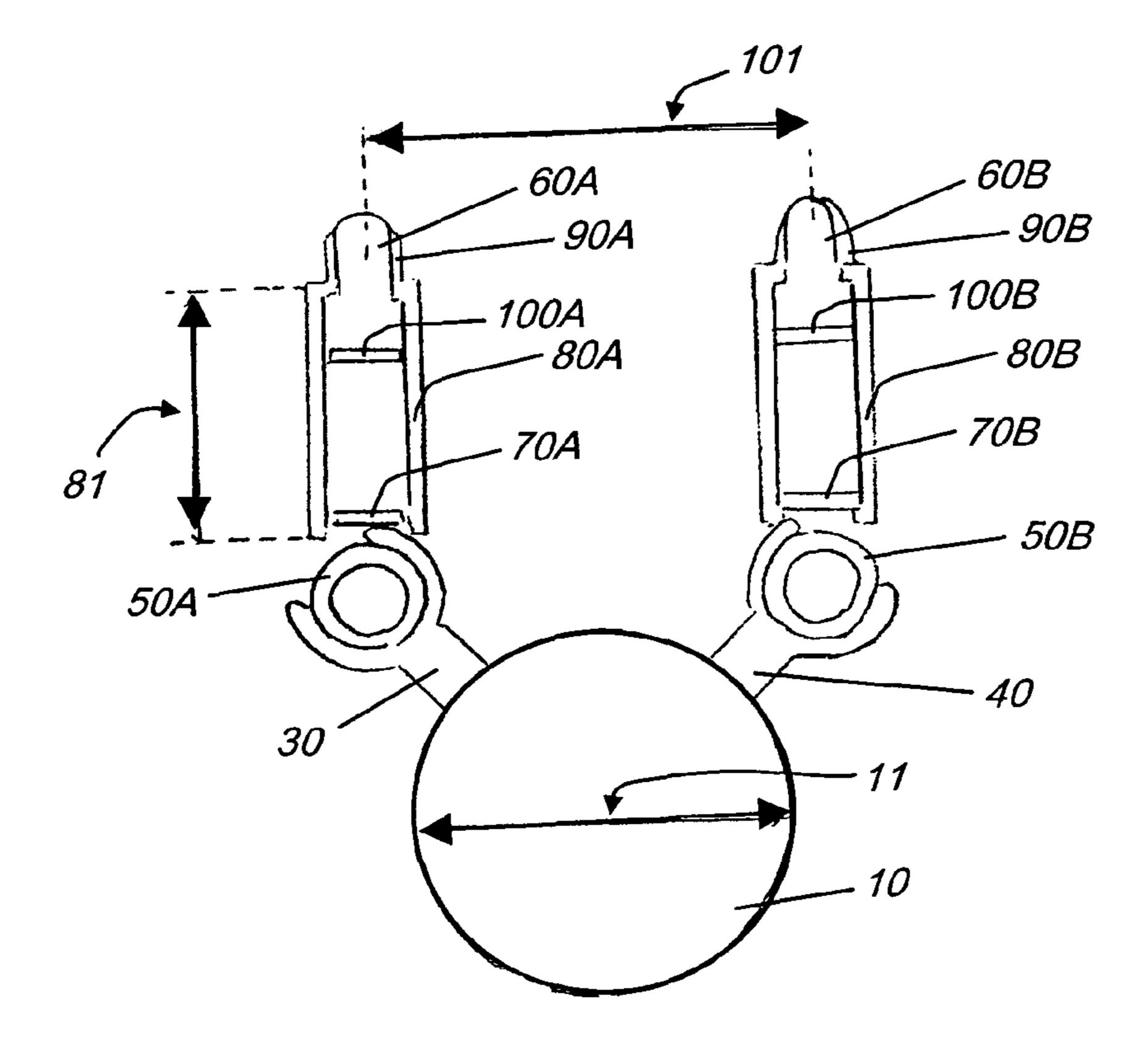
FIGURE 3: Caricature of a view from underneath of an illustrative, non-exclusive embodi-ment of a device according to the invention illustrating relative dimensions of components in one configuration.
