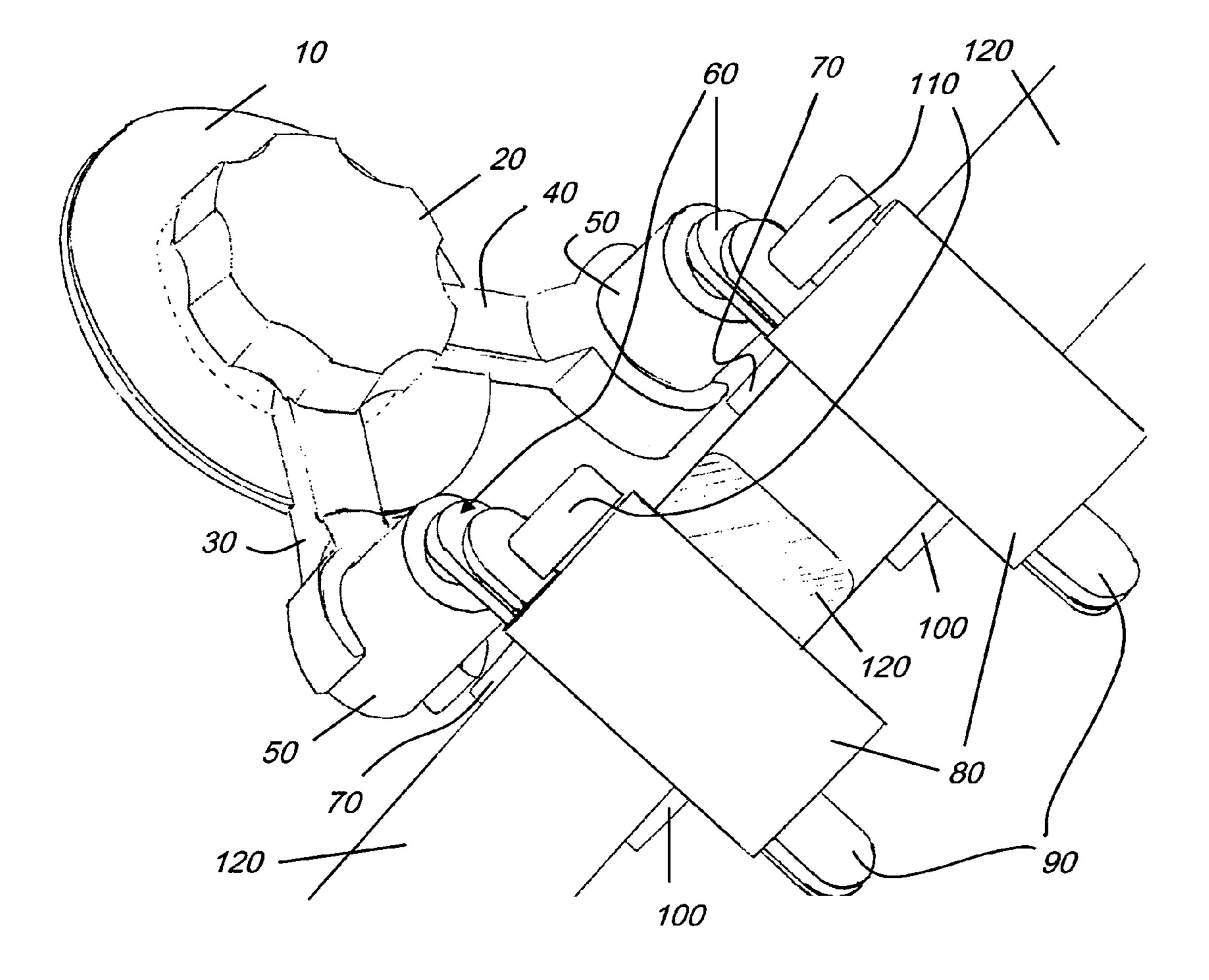
FIGURE 1: Caricature of an upper view of an illustrative, non-exclusive embodiment of a device according to the invention when locking windshield wipers on a vehicle window.
