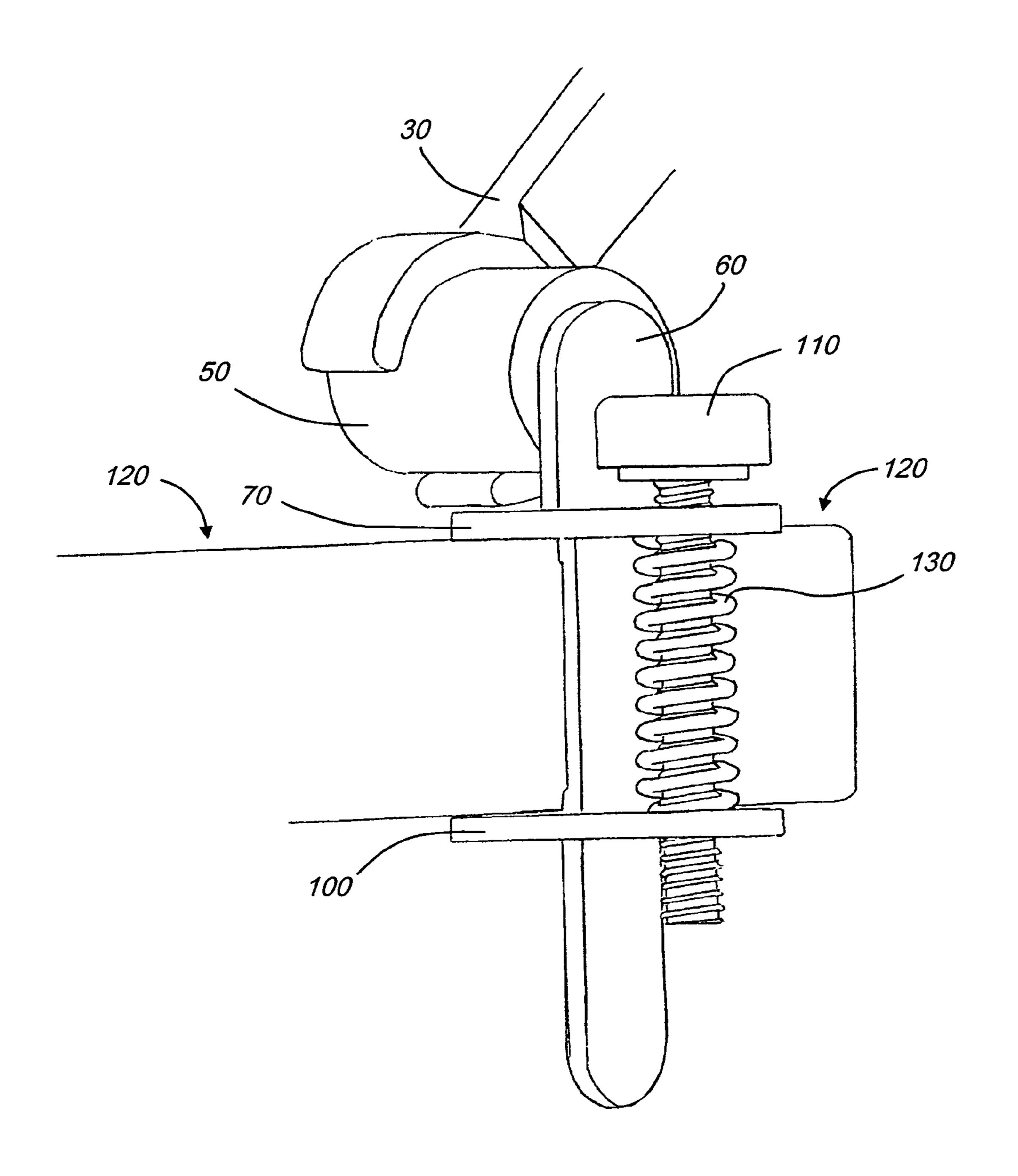
FIGURE 6: Caricature of an upper view of an illustrative, non-exclusive embodiment of a device according to the invention illustrating internal components of a blade lock in one configuration.
