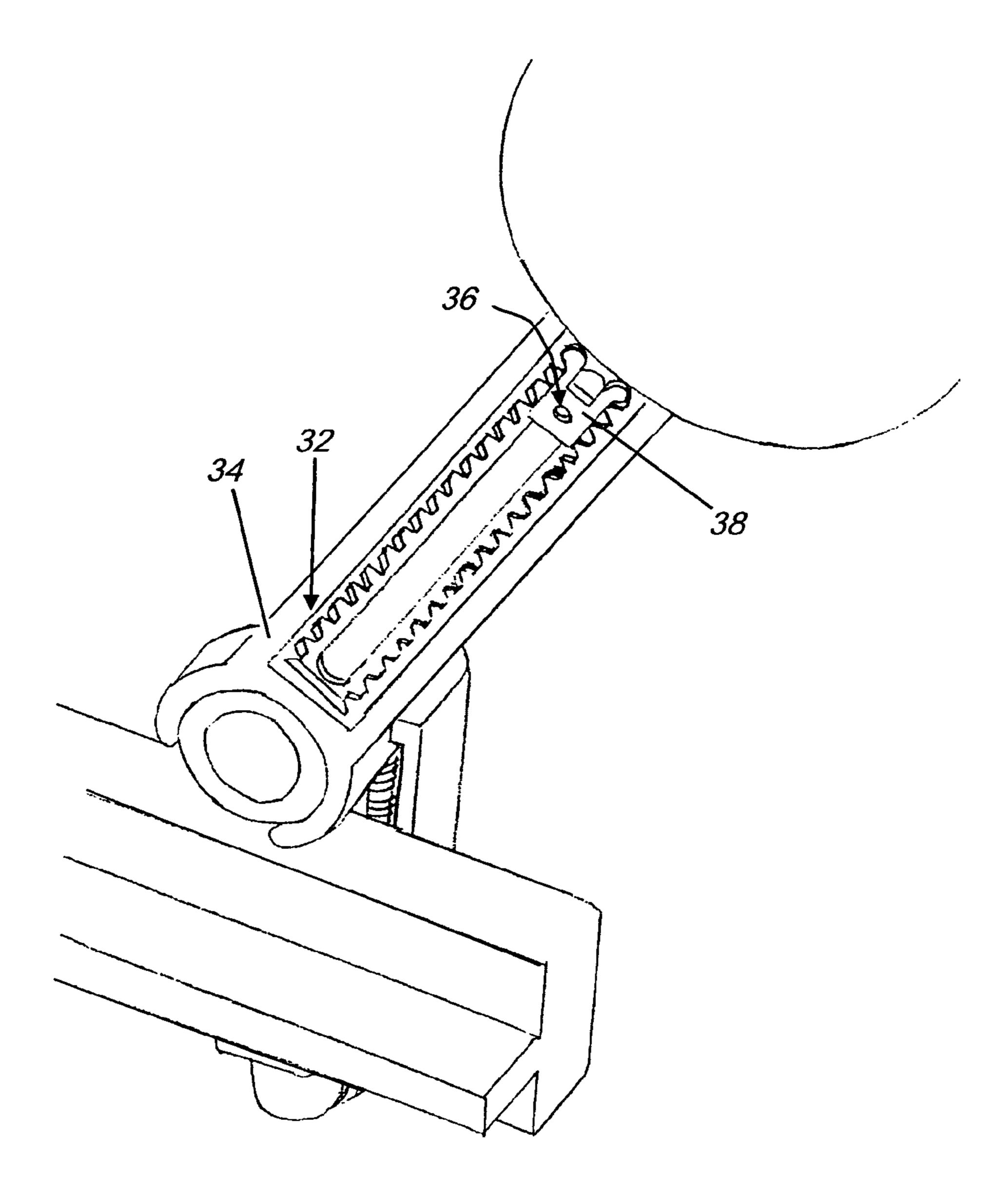
FIGURE 5: Caricature of an upper view of an illustrative, non-exclusive embodiment of a device according to the invention illustrating additional aspects of an extendible arm in one configuration.
