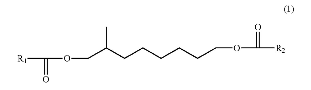
The lubricating oil base oil is suitable for a fluid dynamic pressure bearing, an oil-impregnated porous bearing, or a dynamic pressure-type oil-impregnated porous bearing.
