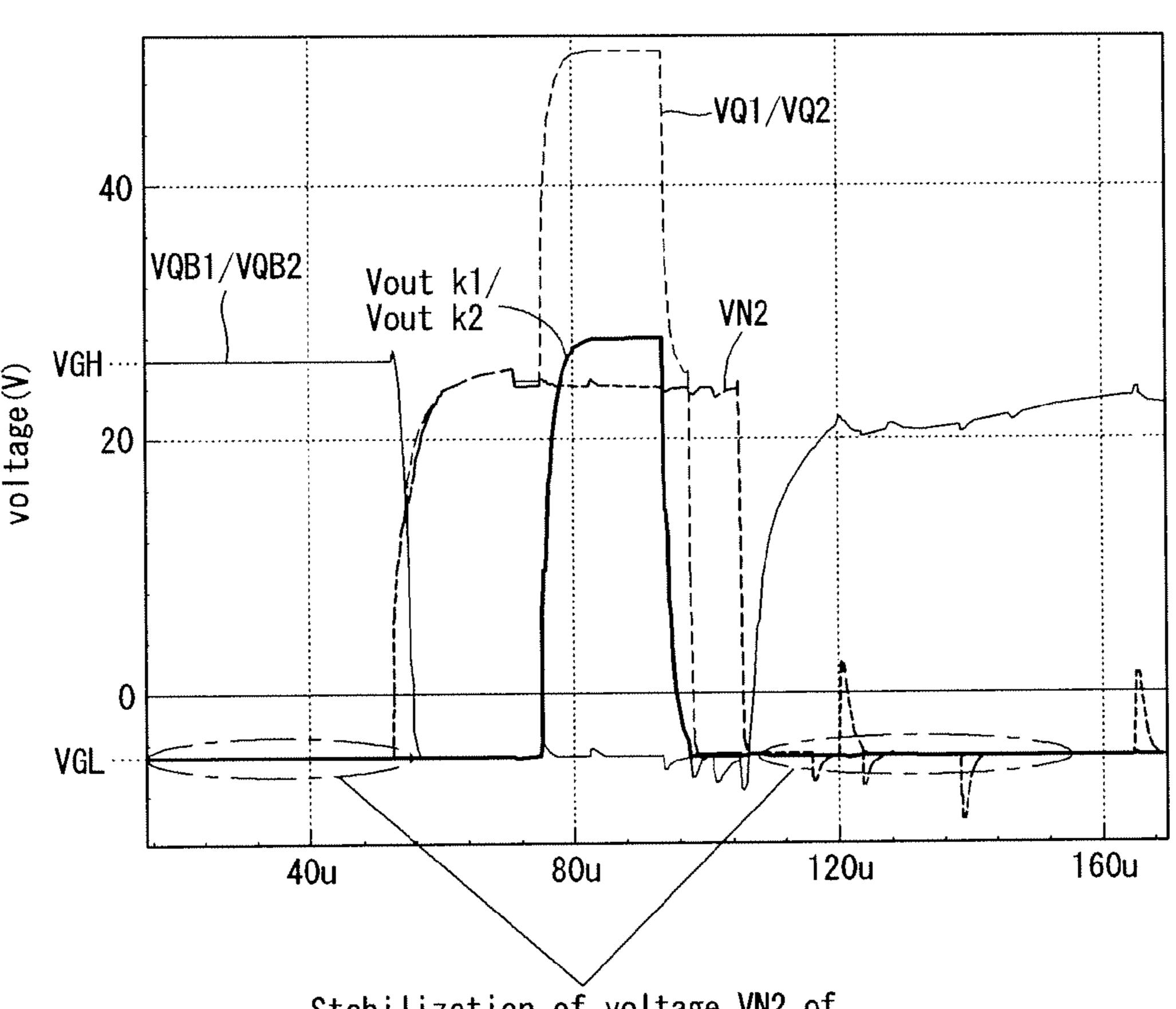
Stabilization of voltage VN2 of second node to gate low voltage VGL
