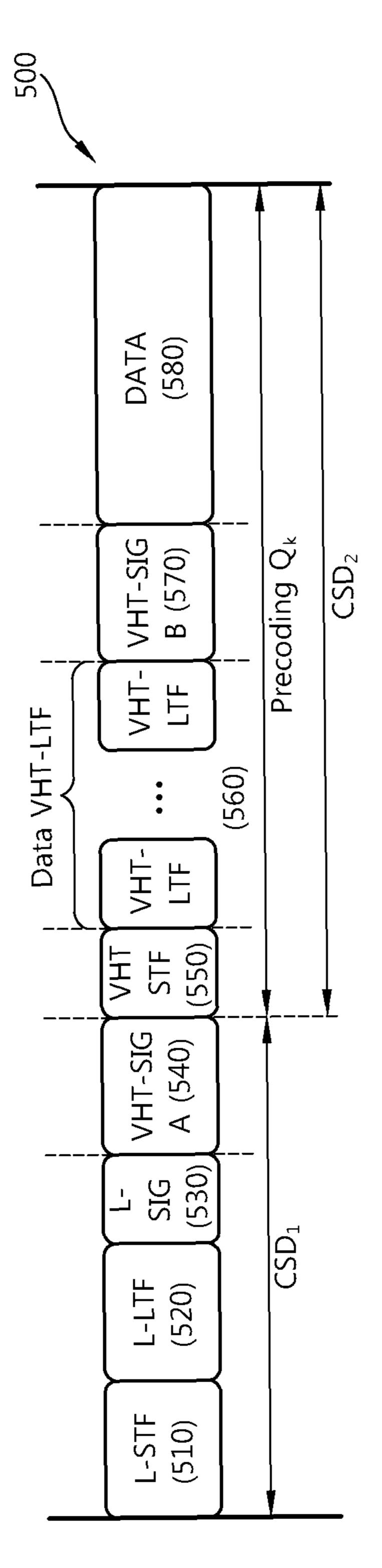
Note :  ${\sf CSD}_1$  is performed at Tx antenna chain domain,  ${\sf CDS}_2$  is performed at spatial stream domain
