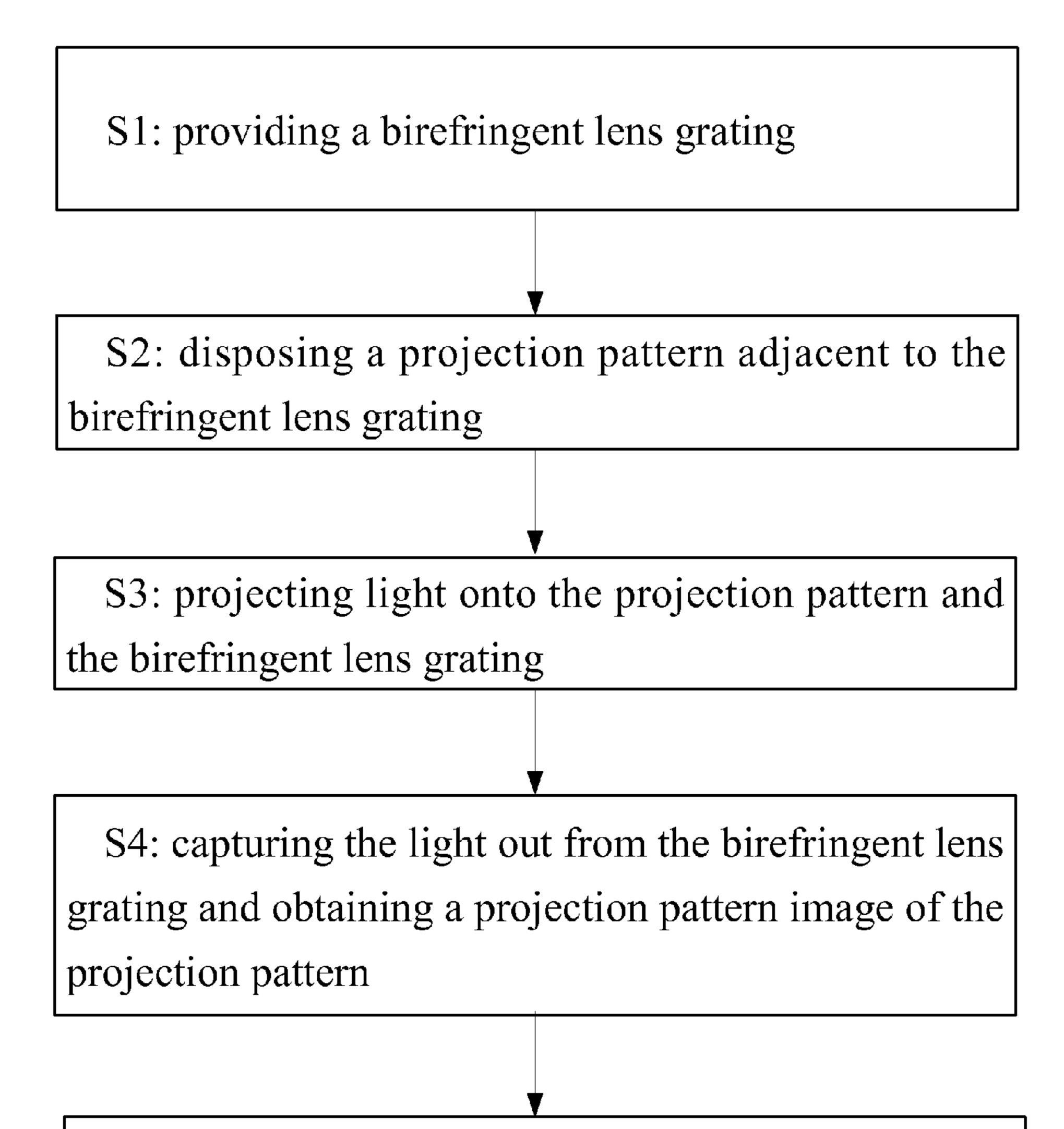
S5: comparing the projection pattern image with a reference to determine a refractive index matching degree of the birefringent lens grating
