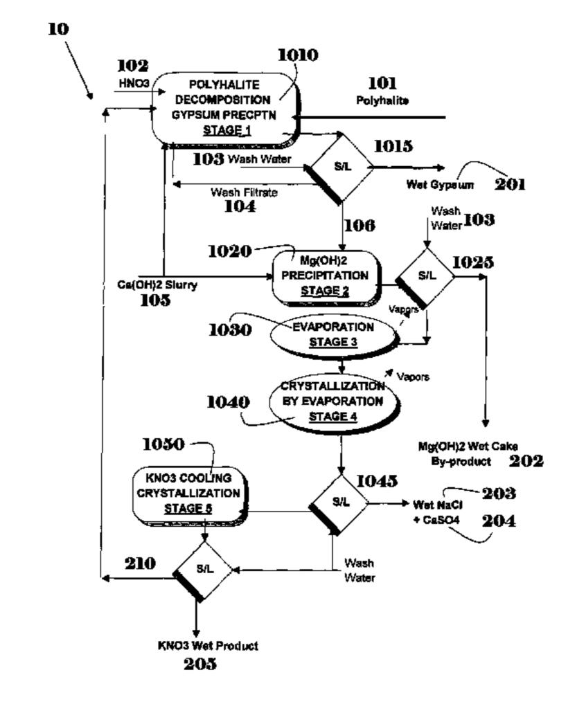
steps of (a) contacting polyhalite with HNO3; (b) adding Ca(OH)2 to the solution, thereby precipitating as CaSO4 at least part of the sulfate present in said solution; (c) precipitating as Mg(OH)2 at least part of the Mg2+ remaining in said solution by further addition of Ca(OH)2 to the remaining solution; (d) concentrating the solution, thereby precipitating as a sulfate compound at least part of the sulfate remaining in solution; (e) separating at least part of the NaCl from the
