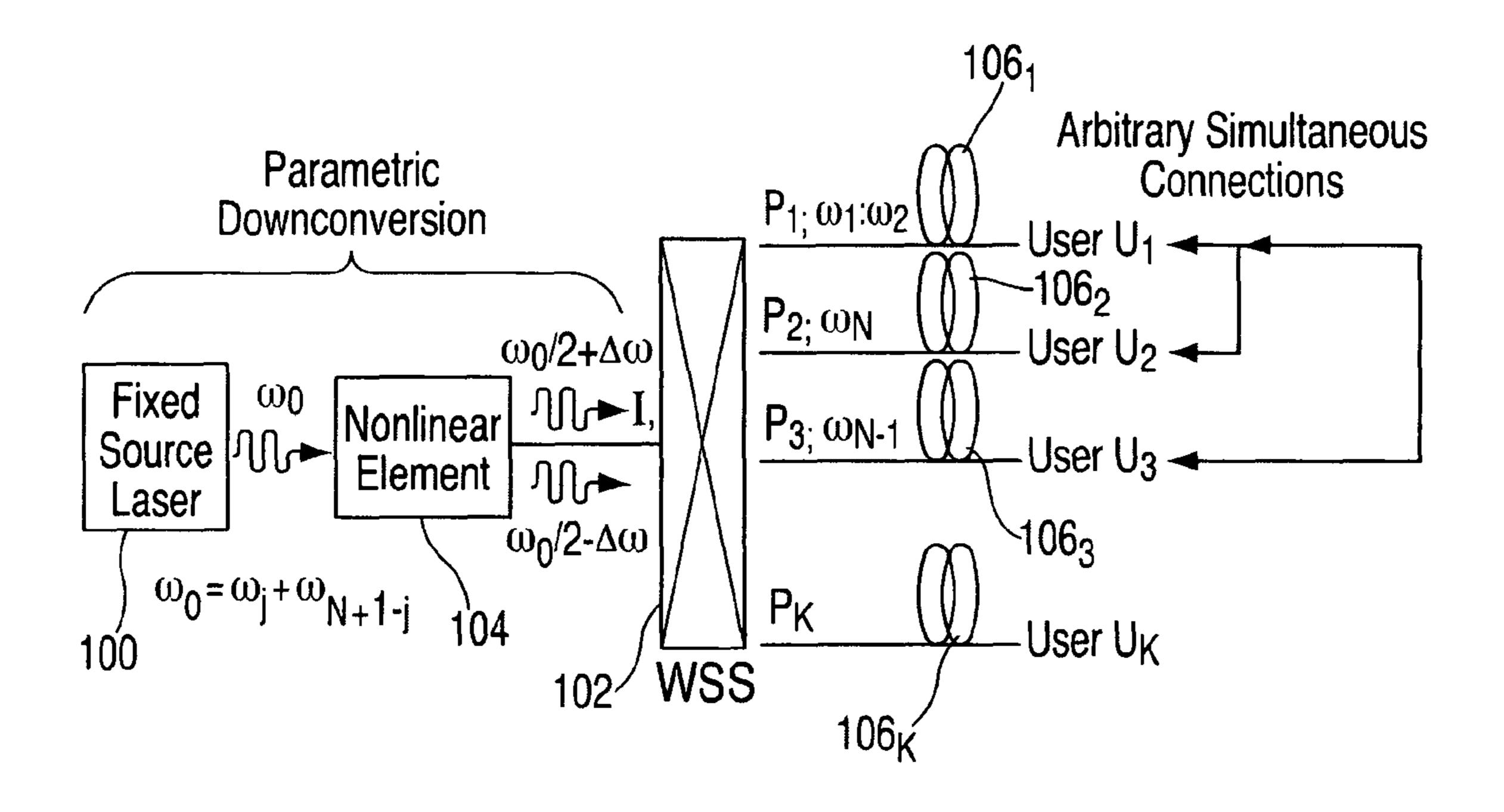
A 1xK wavelength selective switch (WSS) can be used to set up arbitrary simultaneous QKD connections, subject to the limit of total wavelength count.
