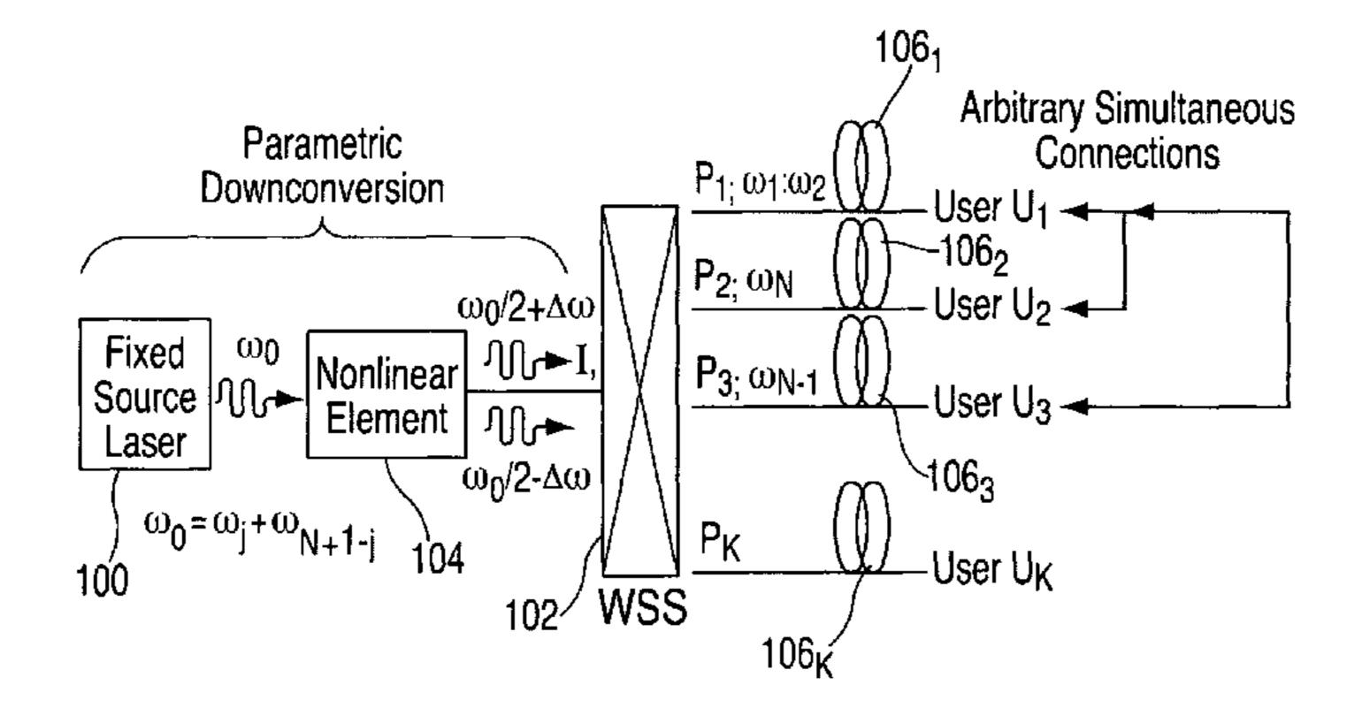
A 1xK wavelength selective switch (WSS) can be used to set up arbitrary simultaneous QKD connections, subject to the limit of total wavelength count.
