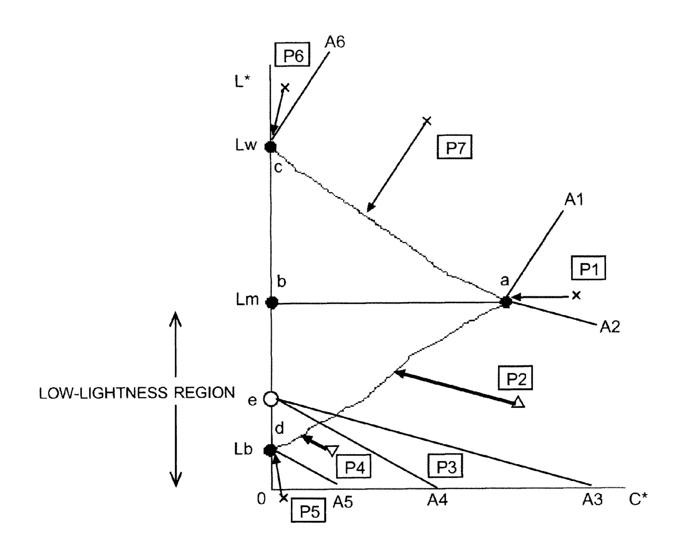
e(O): ADJUST POSITION OF REFERENCE POINT e IN DIRECTION Lb BECAUSE OF SMALL LIMITING VALUE OF TOTAL QUANTITY OF COLOR MATERIAL
