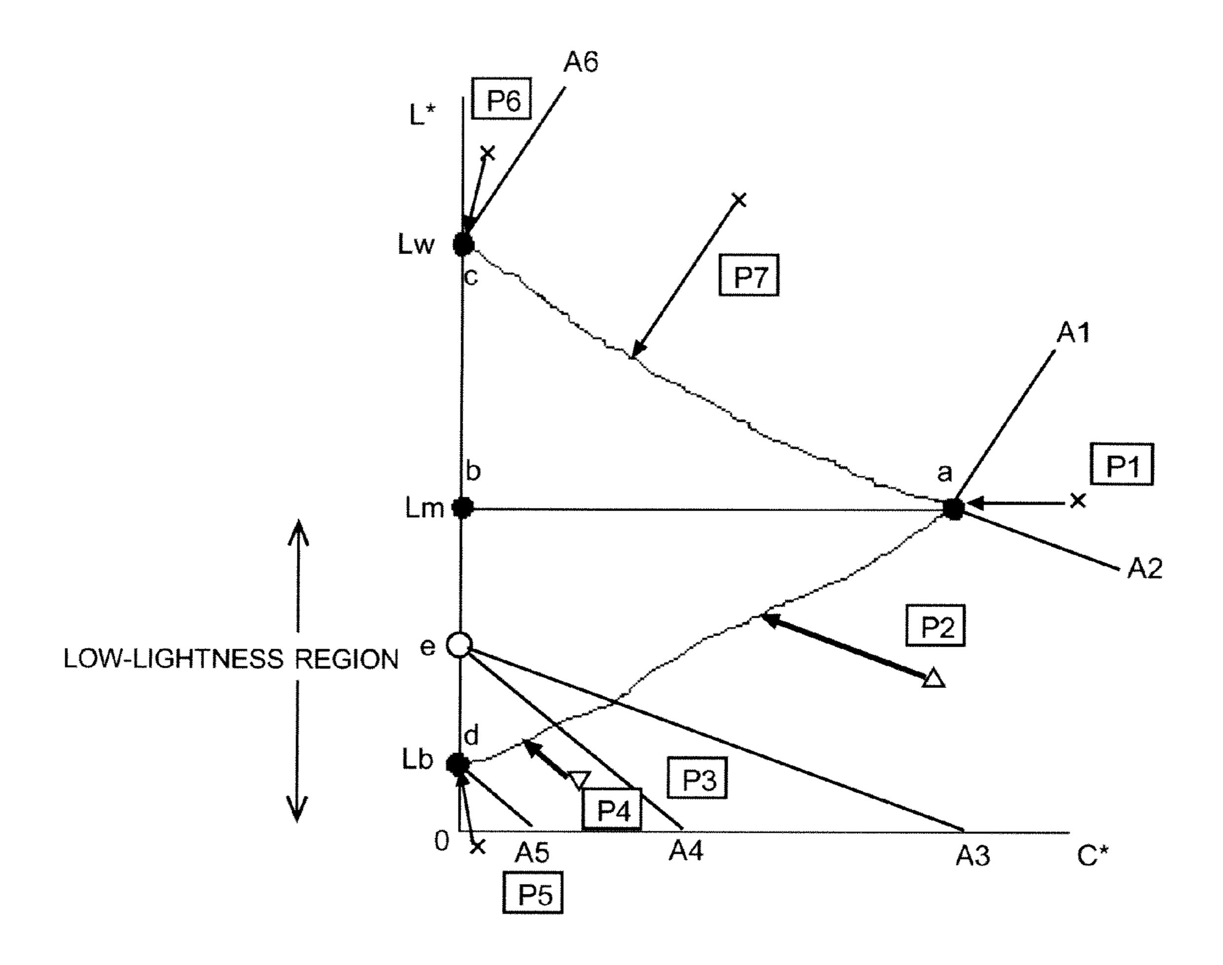
e(O) :ADJUST POSITION OF REFERENCE POINT e TOWARD Lb BECAUSE OF SMALL LIMITING VALUE OF TOTAL QUANTITY OF COLOR MATERIAL :CHANGE GAMUT-MAPPING ANGLE BASED ON LIMITING VALUE OF TOTAL QUANTITY OF COLOR MATERIAL TO REDUCE ITS SLOPE
