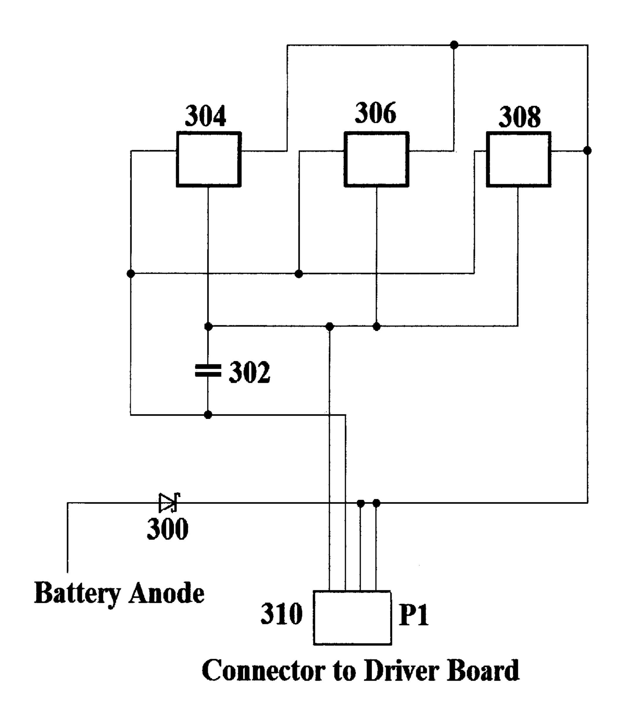
Fig. 4 – Schematic that shows one embodiment for a flashlight LED circuit
