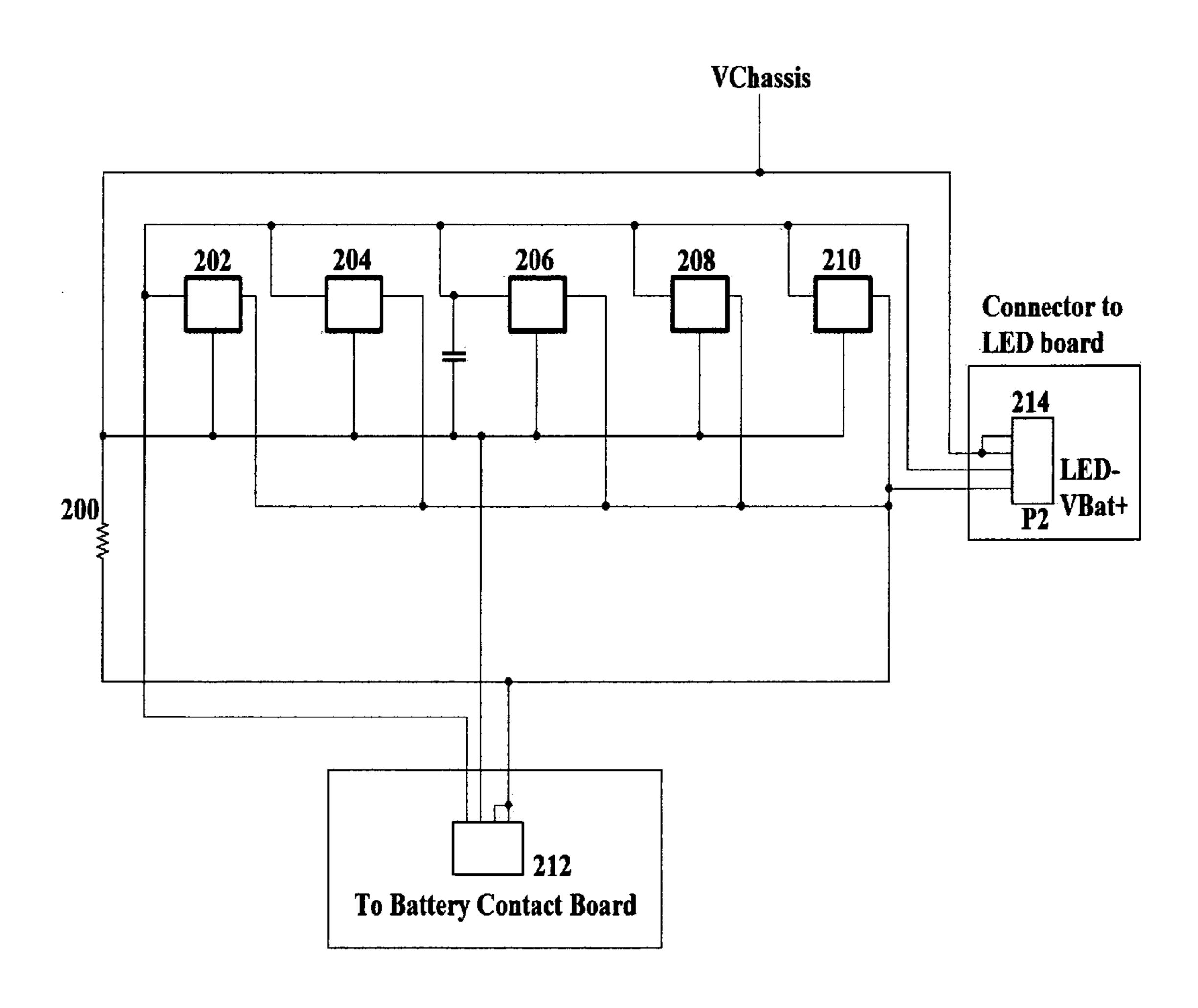
Fig. 3 – Schematic that shows one embodiment for a flashlight battery contact circuit
