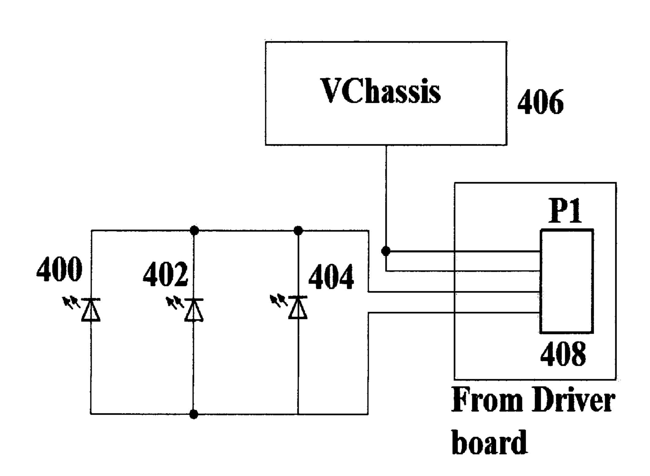
Fig. 1 – Schematic that shows one embodiment of a powered tail cap circuit that implements a directional switch and inertial sensor.
