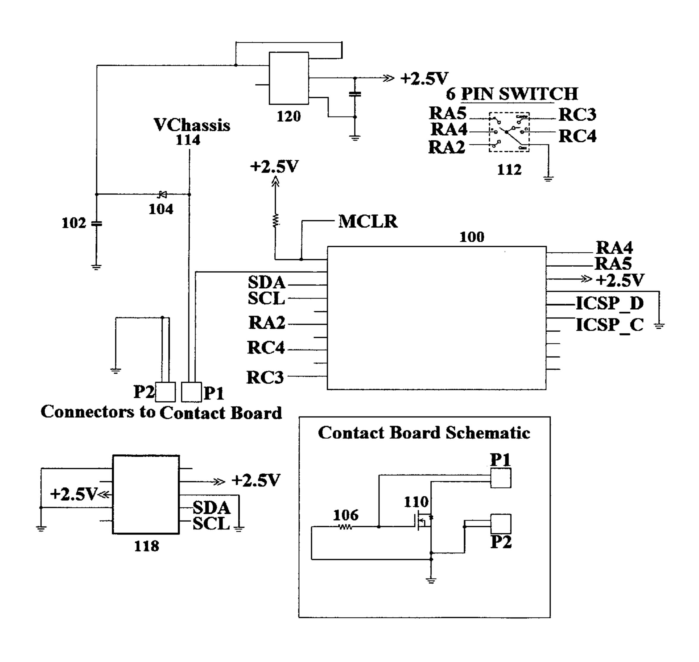
Fig. 2 – Schematic that shows one embodiment for a flashlight driver circuit
