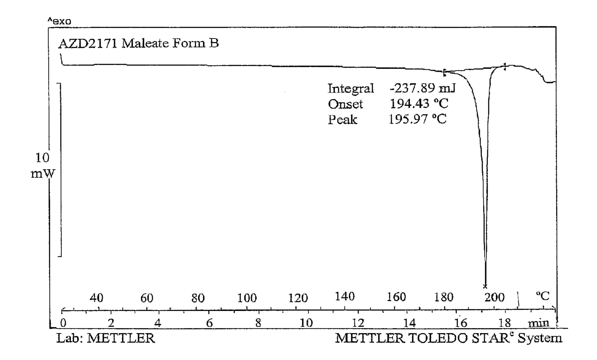
Figure 9: DSC Thermogram AZD2171 Maleate Form B
