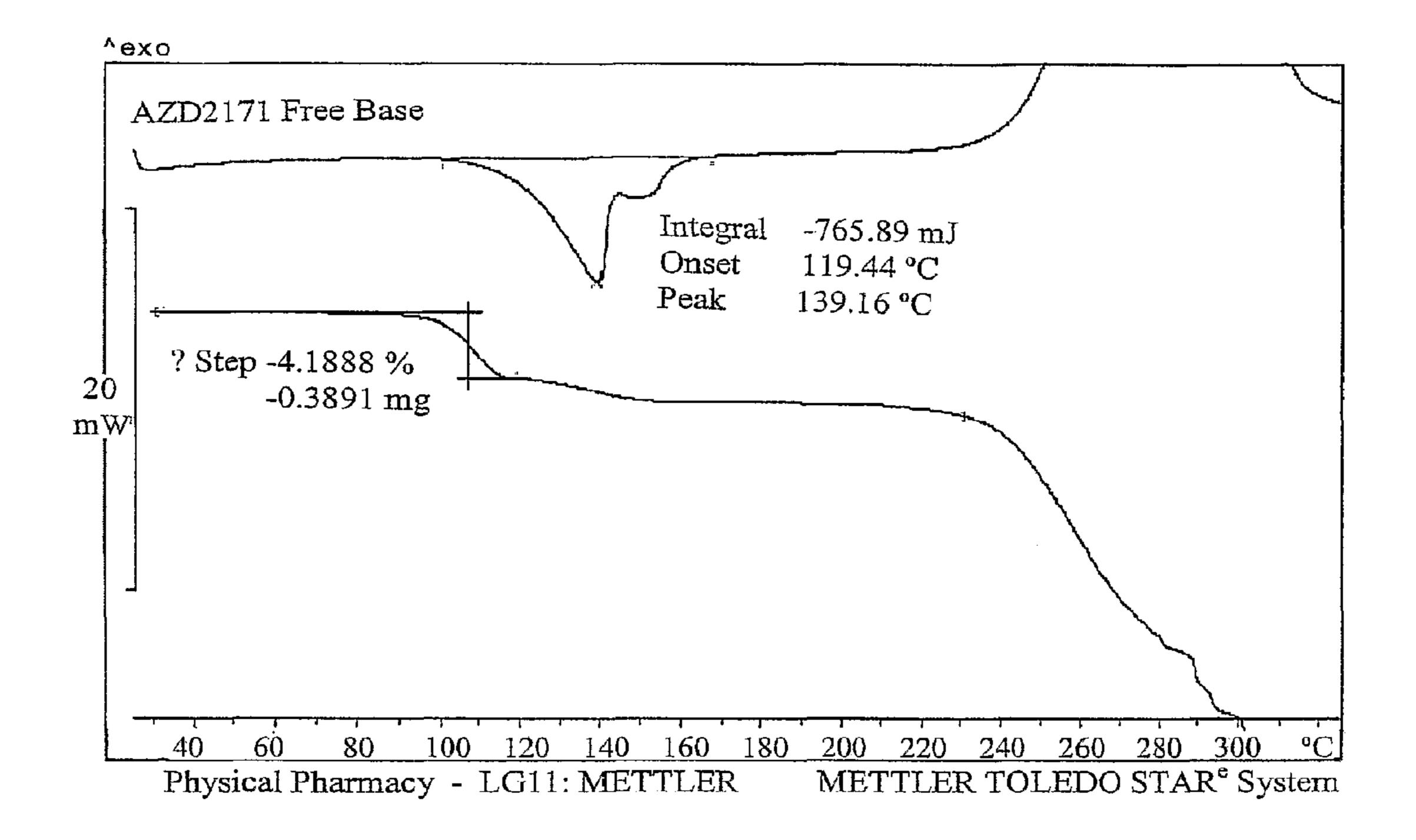
Figure 1: DSC and TGA Thermograms AZD2171 Free base Monohydrate
