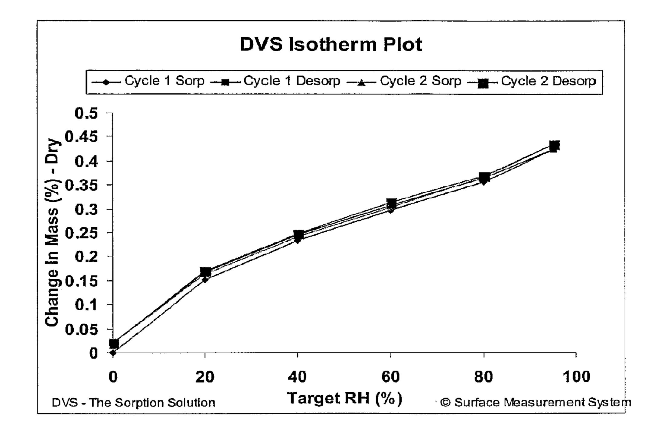
Figure 7: AZD2171 Maleate Form A Vapour Sorption Isotherm at 25° C
