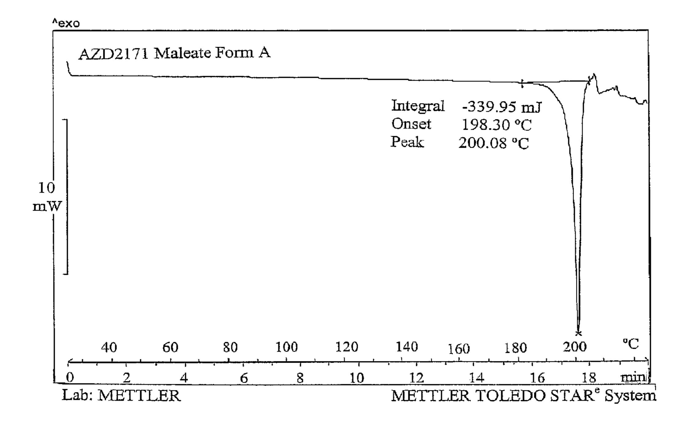
Figure 6: DSC Thermogram AZD2171 Maleate Form A
