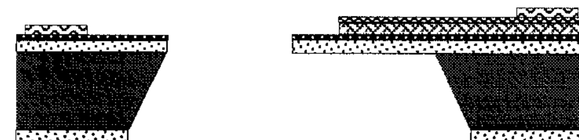
(i) Etch SiO 2 from the front side by RIE to release cantilever
