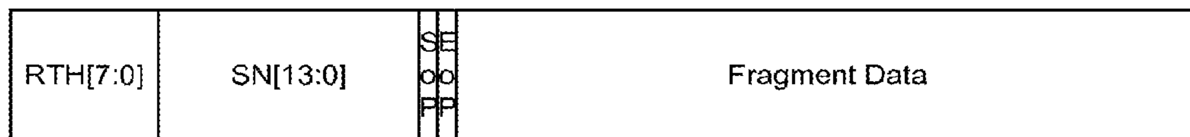
Standardized PAF Fragment with additional Retransmission Header RTH
