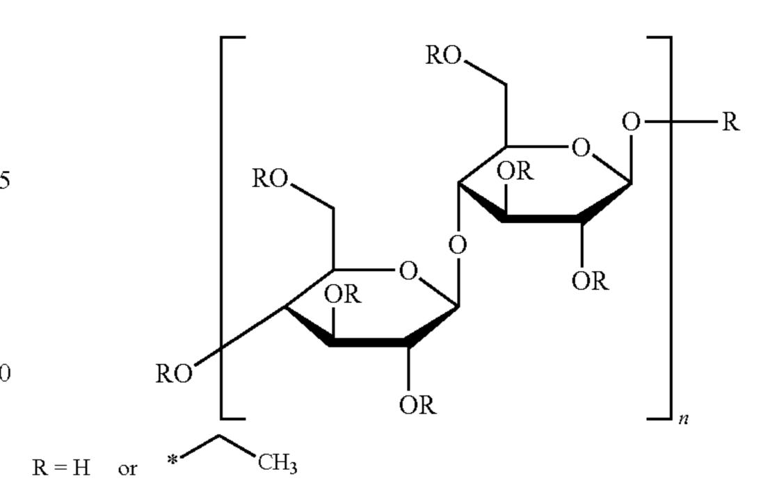
The degree of substitution of the ethylcellulose preferably used in the present invention is preferably between 2 and 3, more preferably about 2.5. The average number of hydroxyl groups substituted per anhydroglucose unit (the 'monomer') is known as the 'degree of substitution' (DS). If all three hydroxyls are replaced, the maximum theoretical DS of 3 results.
