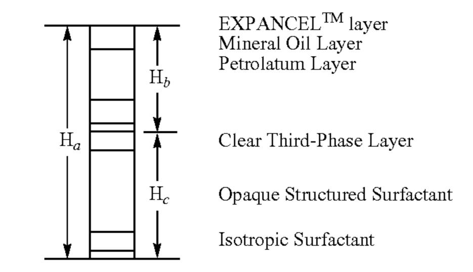
First, the total height is measured as  $H_a$  which includes all materials in the ultracentrifuge tube. Second, the height of the benefit layer is measured as  $H_b$ . Third, the structured surfactant layer is measured as H. The benefit layer is determined by its low moisture content (e.g. less than 10% water as measured by Karl Fischer Titration). It generally presents at the top of the centrifuge tube.
