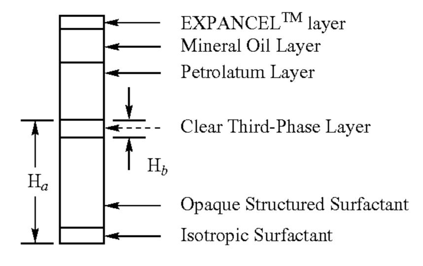
When a density modifier such as EXPANCEL<sup>TM</sup> low density microspheres is used, the very top layer primarily comprises the EXPANCEL<sup>TM</sup> low density microspheres. The second layer from the top is the clear mineral oil layer. The third layer from the top is the petrolatum layer. The layers below 65 the petrolatum layers contain aqueous surfactant and are characterized as follows: H<sub>a</sub> is the height of all the aqueous and/or
