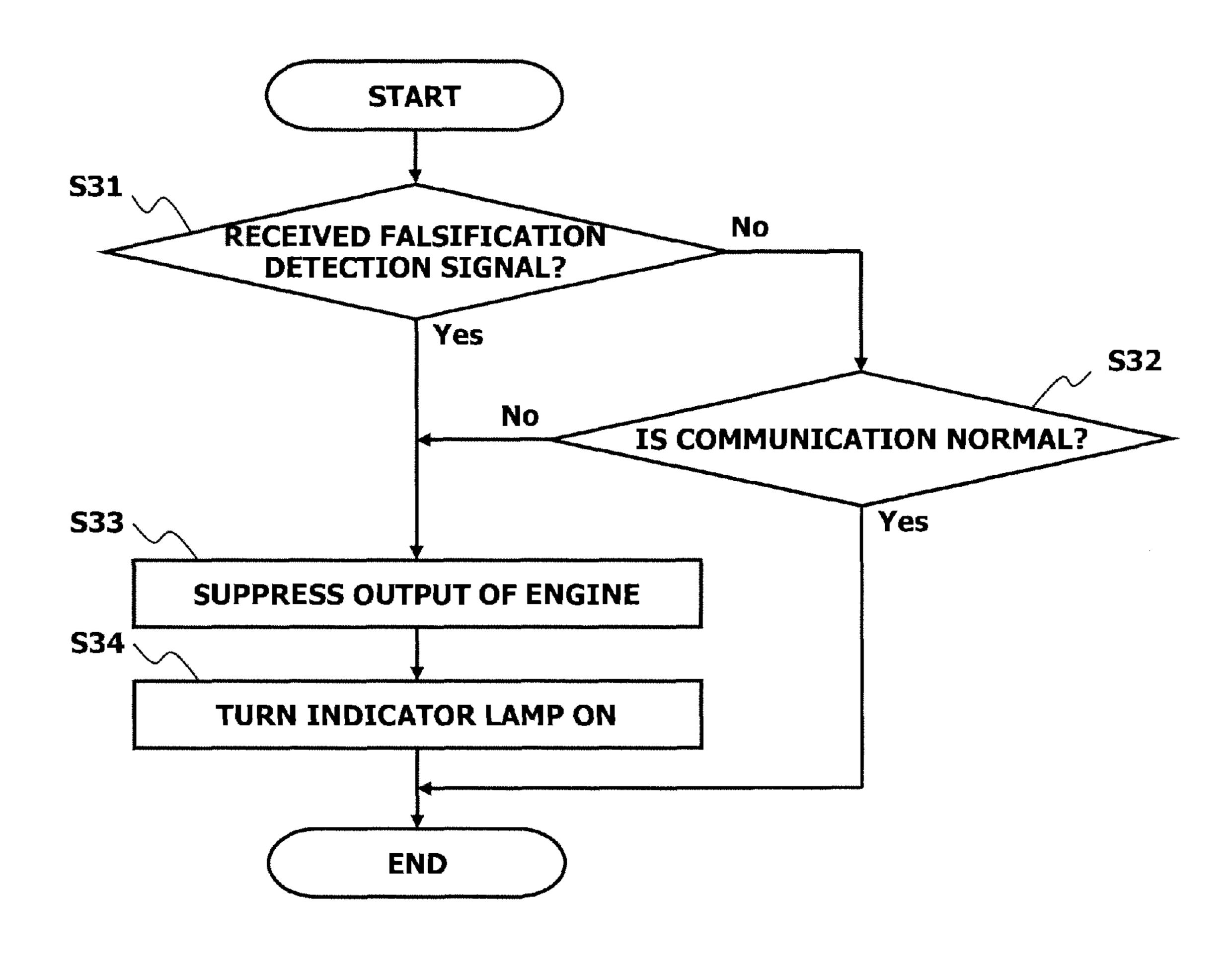
VEHICLE SPEED SIGNAL FALSIFICATION
