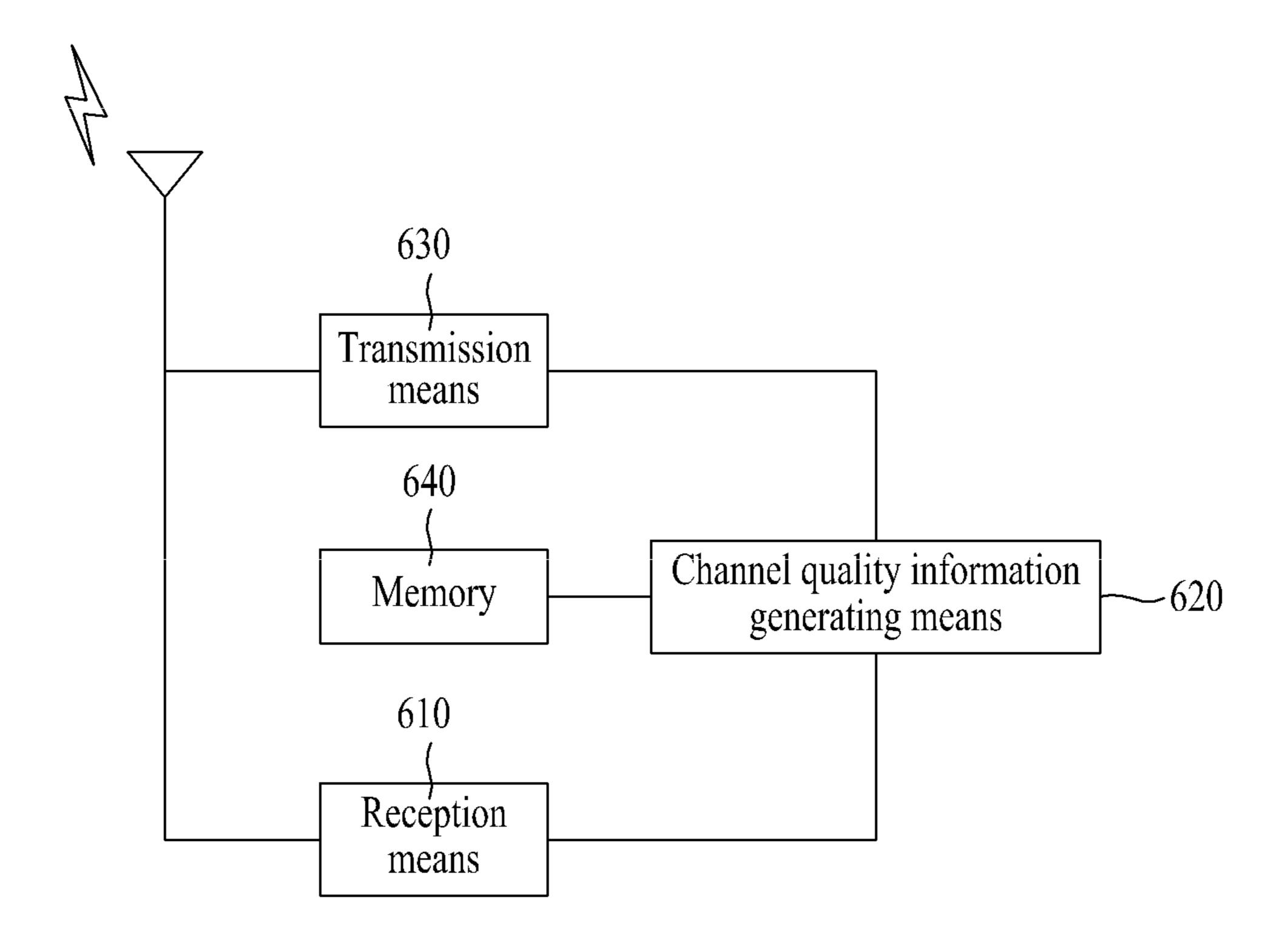
METHOD FOR TRANSMITTING FEEDBACK INFORMATION IN COMP, TERMINAL FOR PERFORMING SAME, METHOD FOR GENERATING CHANNEL STATE INFORMATION AND BASE STATION APPARATUS FOR PERFORMING SAME
