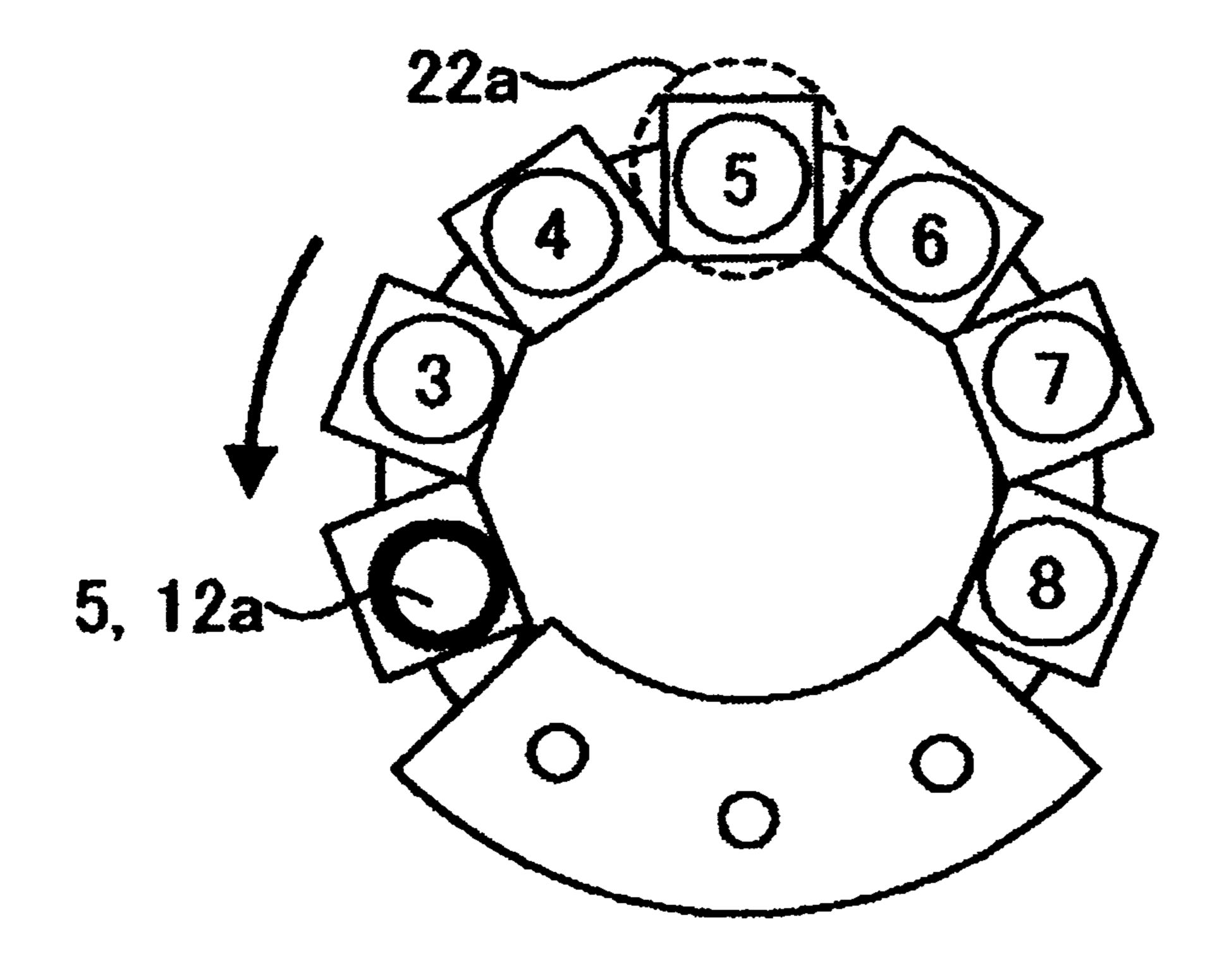
(4) CAUSE THE STOPPER BODY 5 TO STAND BY, AND HOLD THE STOPPER BODY 5
