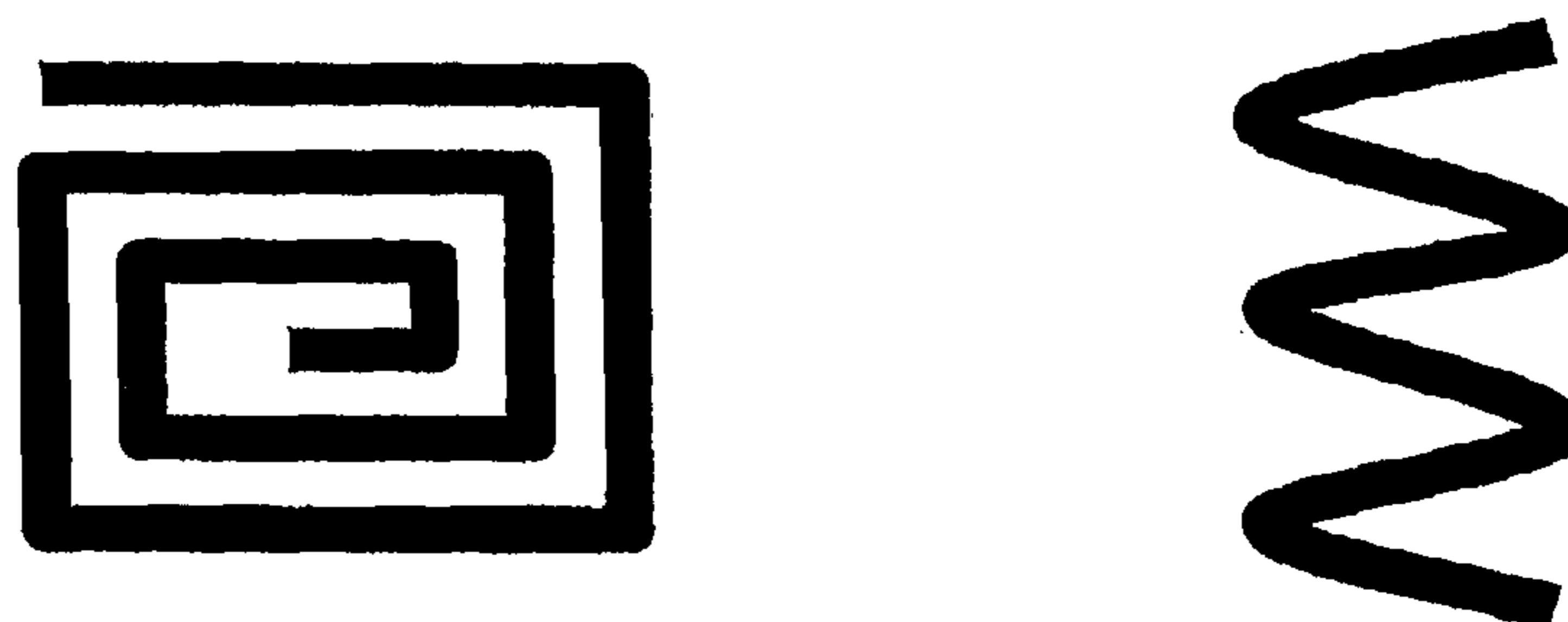
Figure 2: Schematic forms of antenna structures in thin strip form (rectangular cross-section). For illustrative purposes only.
