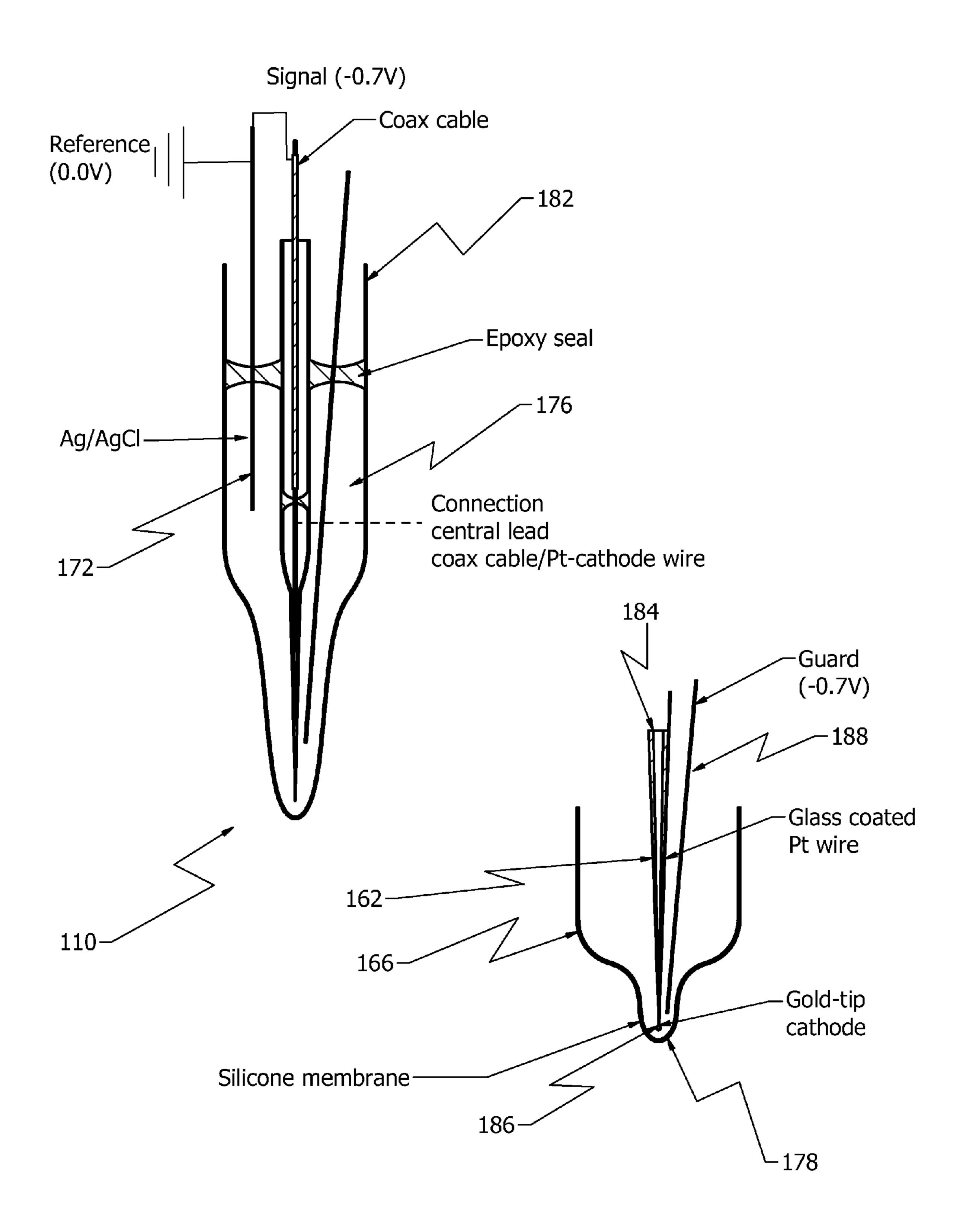
Figure 1F - shape of the 02 microelectrode
