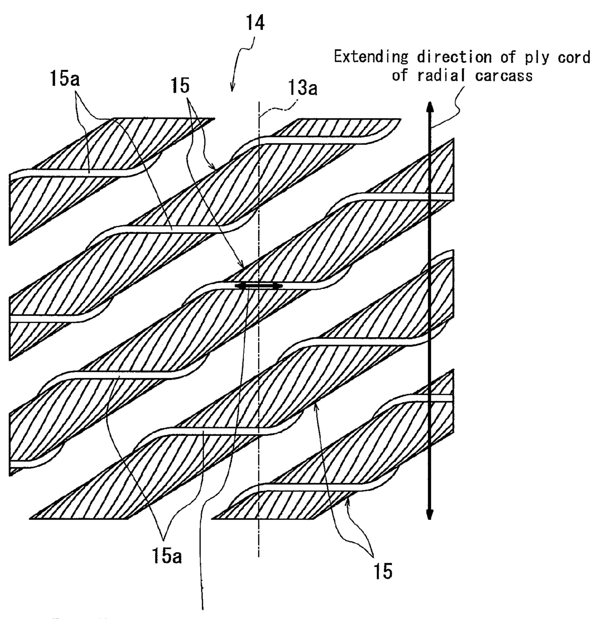
Extending direction of spiral filament 15a
