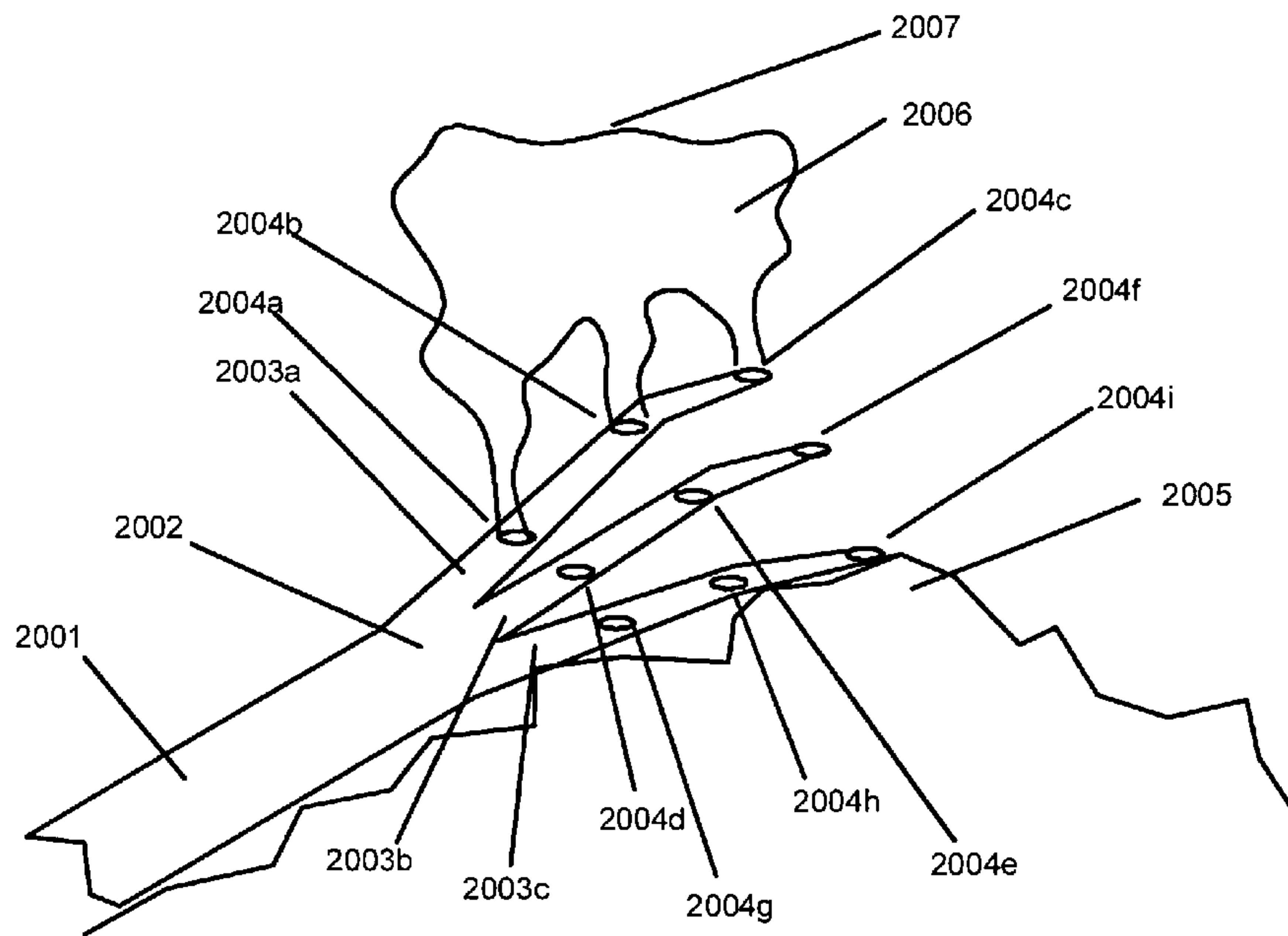
Figure 20: A method of releasing moisture-laden air from the top of a chimney
