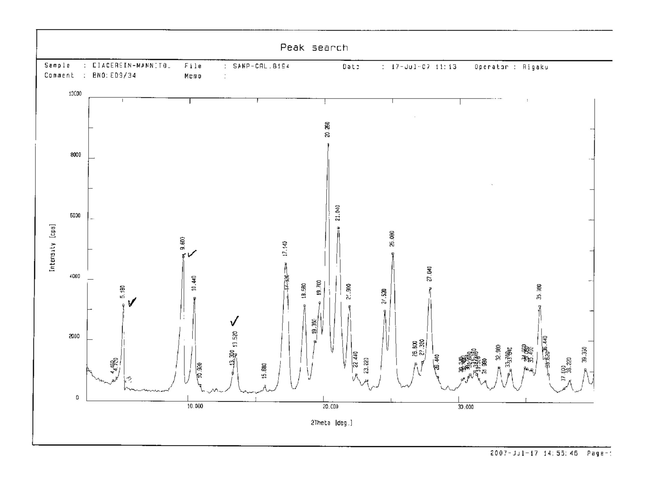
FIGURE 2: X-ray diffraction pattern of plain Diacerein
