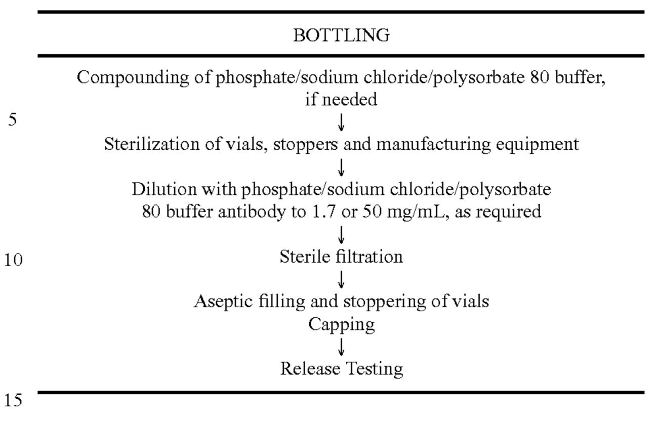
More specifically, natalizumab obtained for example by the procedures discussed above, can be bottled as follows. Natalizumab 200 L and 2000 L drug product can be filled on a fully automated filling line equipped with a vial washing, sterilization and depyrogenation tunnel. Stoppers, seals and filling equipment are washed and sterilized prior to use. This process allows for large scale tilling operations consistent with the volumes produced from the 2000 L fermentation.
