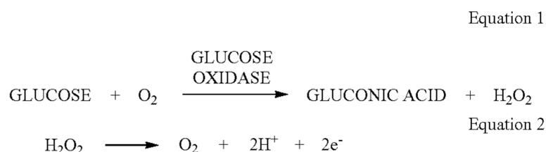
The glucose oxidase is used to catalyze the reaction between glucose and oxygen to yield gluconic acid and hydrogen peroxide (equation 1). The  $\text{H}_2\text{O}_2$  reacts electrochemically as shown in equation 2, and the current can be measured by a potentiostat. These reactions, which occur in a variety of oxidoreductases known in the art, are used in a number of sensor designs.
