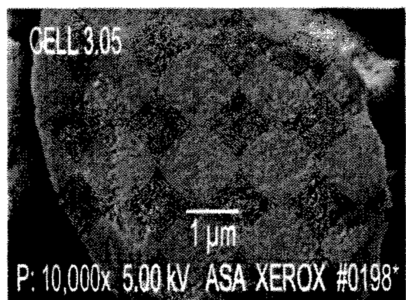
OLD TONER PARTICLE. ADDITIVES HAVE BEEN BEATEN INTO SURFACE
