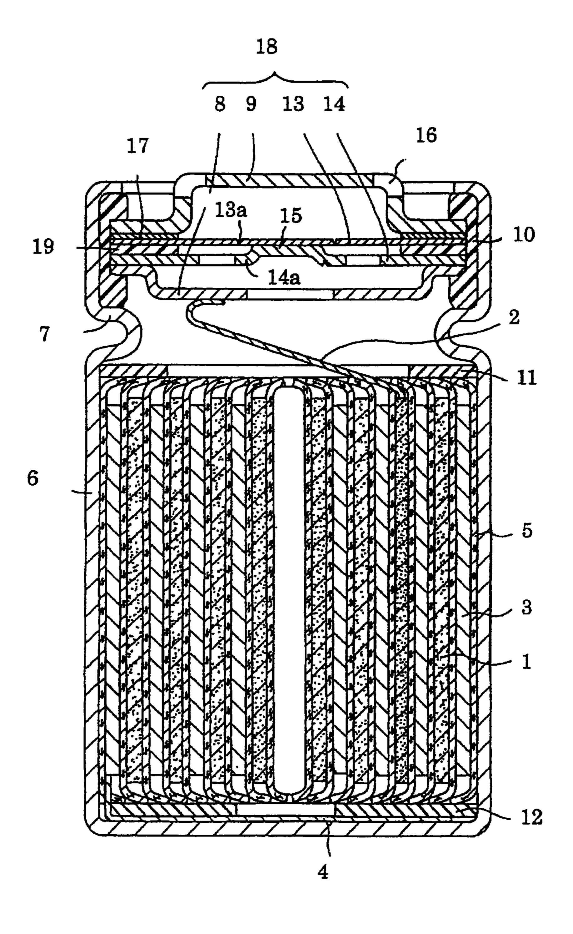
NICKEL HYDROXIDE, METHOD FOR PRODUCING POSITIVE ELECTRODE ACTIVE MATERIAL FOR NON-AQUEOUS ELECTROLYTE SECONDARY BATTERY, ELECTRODE FOR NON-AQUEOUS ELECTROLYTE SECONDARY BATTERY, AND NON-AQUEOUS ELECTROLYTE SECONDARY BATTERY
